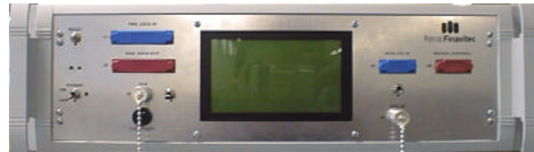
MCE Control Module : - an ERC32 based computer
