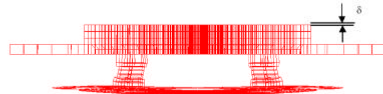
Add-on mirror thermal deformation analysis
