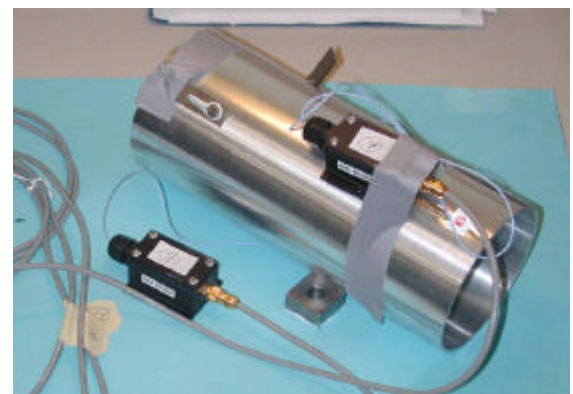
Figure 10: Demo (rocket motor): stress sensor; O 2 sensor; RF-based temp sensor; Fibre Bragg (T, stress, strain)
