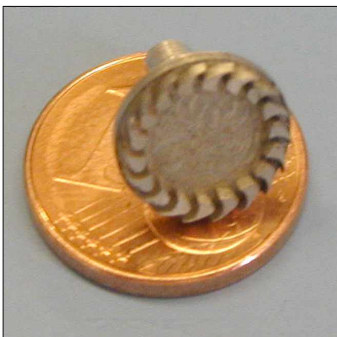
Fig. 6 – Turbo-Bipropellant Microrocket Engine Sketch and first components prototypes
