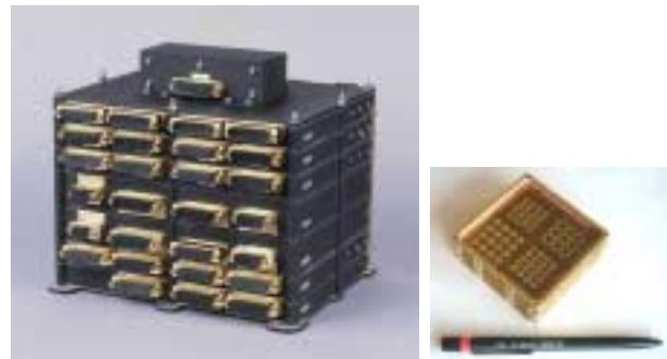
*Figure 17: Left: CON Unit of SMART-1, State of the Art design. Total of ~ 200 ICs, mass: 9.2 kg, dimensions: 259x286x208 mm. Right: 3 MMS Modules includes all components of the CON unit and also discrete components, resistors, capacitors, etc. Total weight: ~120g, size: 74x74x22 mm. Reduction: 70 times in weight, 120 times in volume.*
