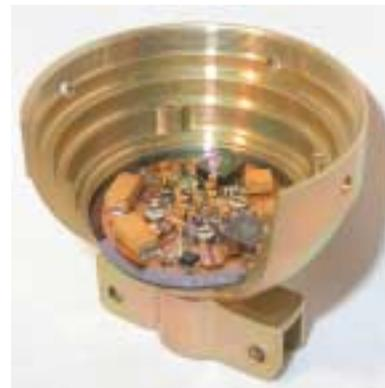
Figure 5: The particle filter stack with the input EMI-filter and double electronic system for conversion of the input voltage to operation voltage for the thruster pod. The 1/4 part of this pod half is cut out for visibility.
