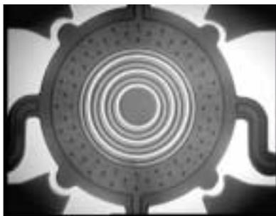
Figure 14: The PCM-valve. The corrugated membranes enclosing the paraffin.
