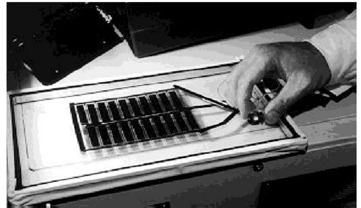
A large area plastic solar cell running a small motor
