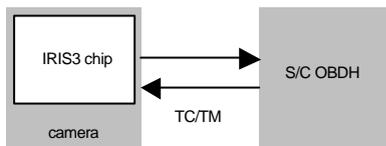
figure 5 Single-chip camera
