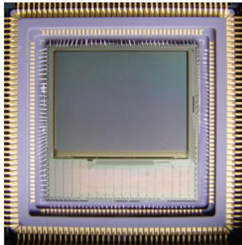
figure 8 IRIS3 camera chip in its QFP package
