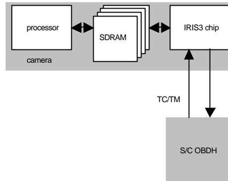
figure 7 Camera with image memory and processor
