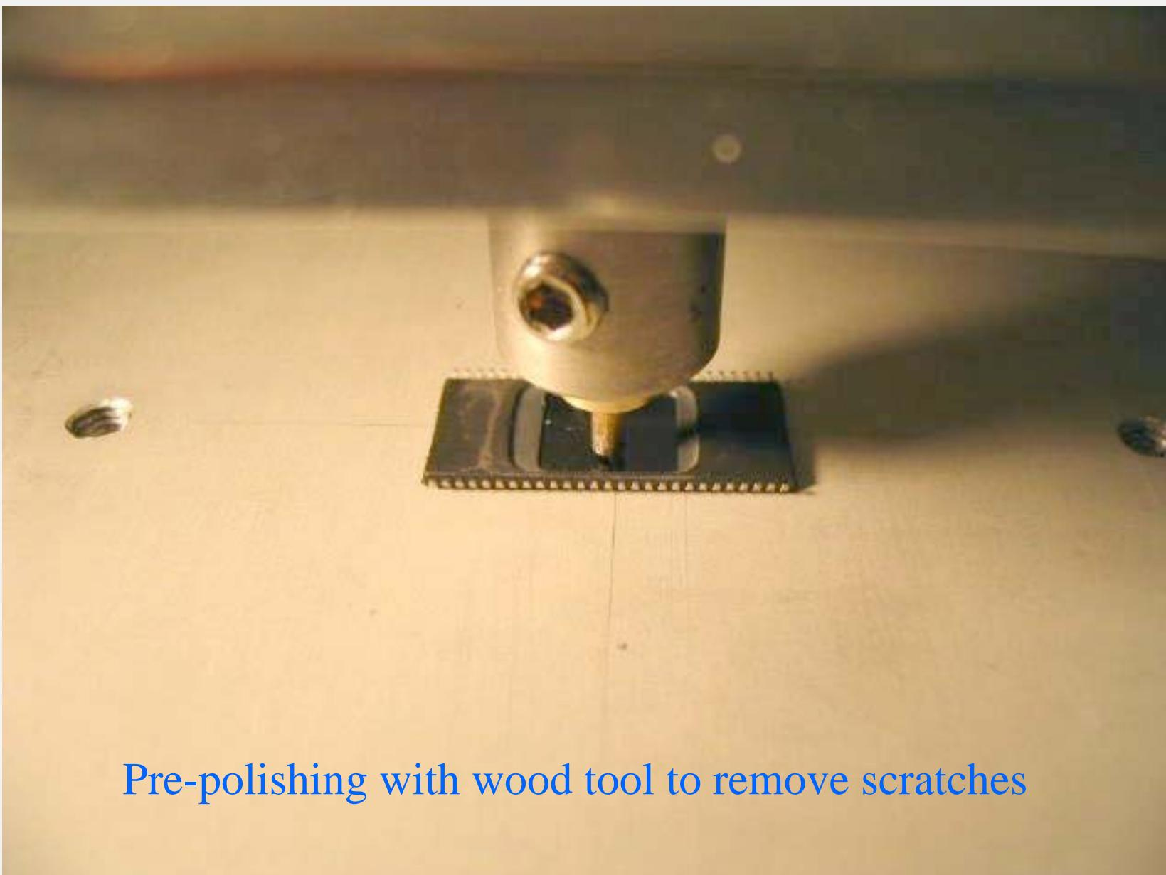
Pre-polishing with wood tool to remove scratches
