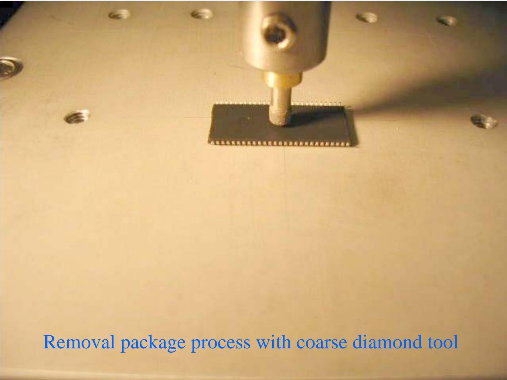
Removal package process with coarse diamond tool
