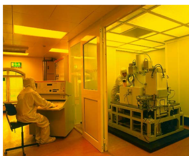
Jeol 6000FS Electron Beam Lithography system with 20nm resolution
