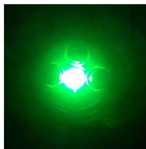
GaN RCLED emitting at 530nm for POF applications
