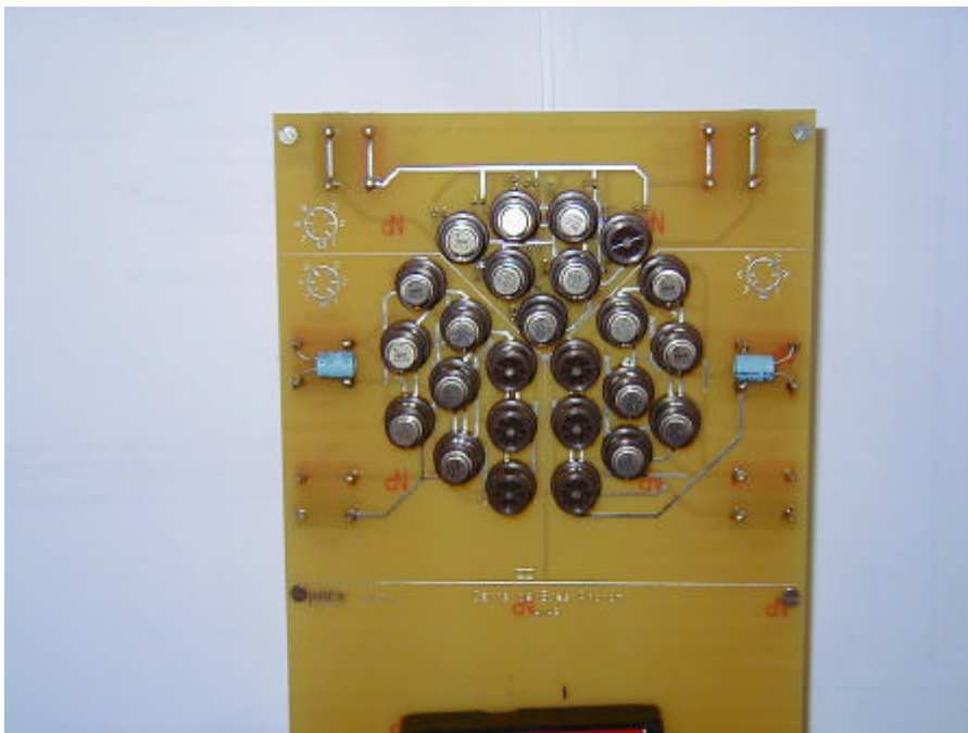
Figure 2 : Photo of the Irradiation Test Board
