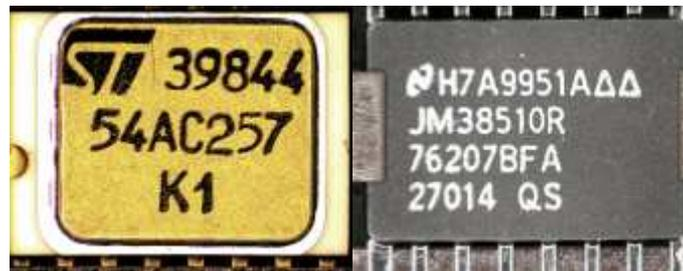
Fig 3.5.2 Picture of the top side of the packages for 54AC257 from STM and 54AC257 from NS
