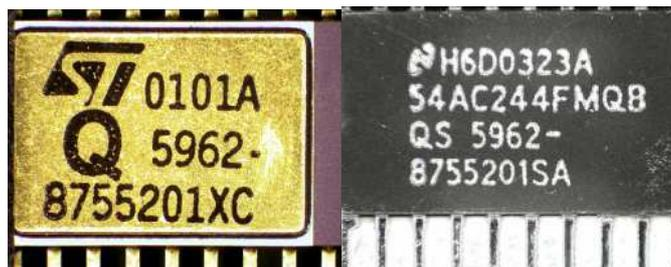
Fig 3.4.2 Picture of the top side of the packages for 54AC from STM and 54AC from NS
