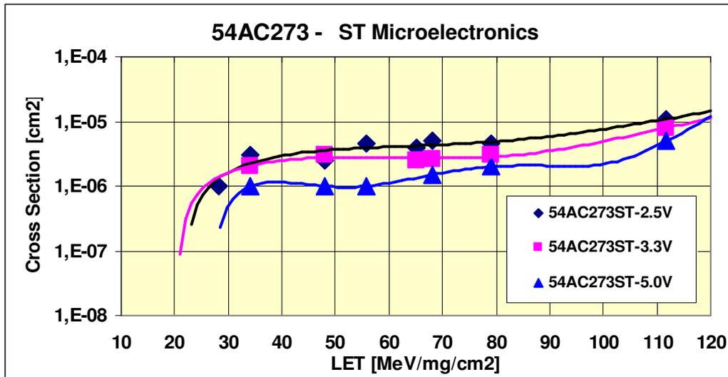
Figure 4.2.2 . Cross Section versus LET value for 54AC273 from ST Microelectronics. The graph shows the average results of two tested devices.
