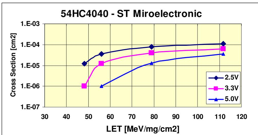
Figure 4.2.4 Cross Section versus LET value for 54HC4040 from ST Microelectronics. The graph shows the average results of two tested devices. The test results for 5V was zero at LET=48.1 MeV/mg/cm<sup>2</sup> and zero for 2.5V at LET=34 MeV/mg/cm<sup>2</sup>.
