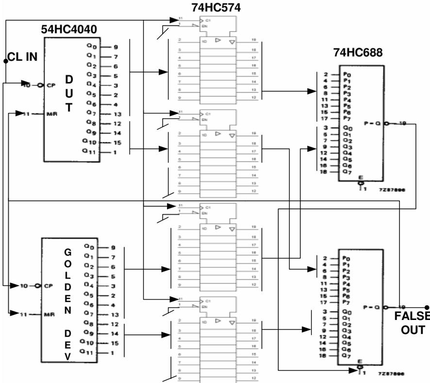
Fig 3.7.1 Test configuration diagram of 54HC4040
