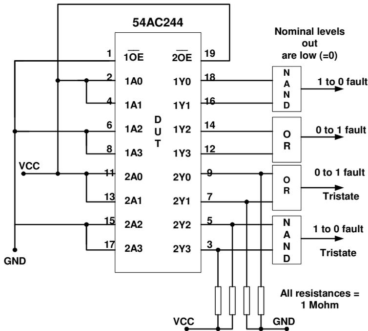
Fig 3.4.1 Test configuration diagram of 54AC244
