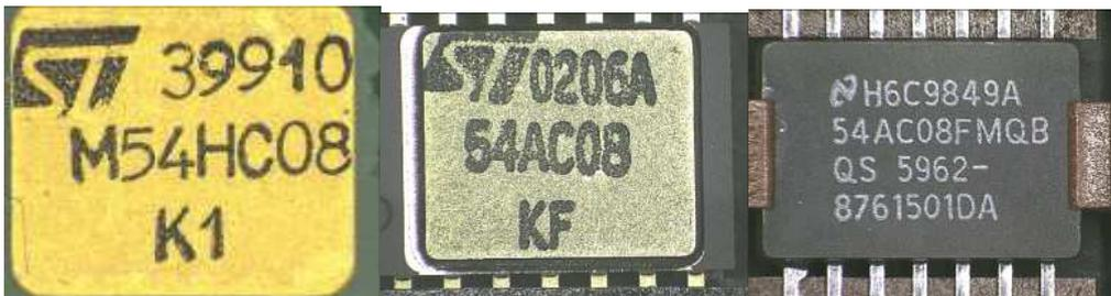
Fig 3.2.2 Picture of the top side of the packages for 54HC from STM. 54AC from STM and 54AC from NS
