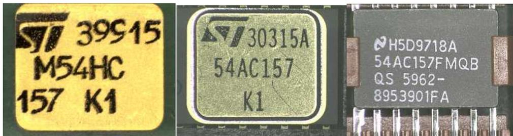
Fig 3.3.1 Picture of the top side of the packages for 54HC from STM, 54AC from STM and 54AC from NS
