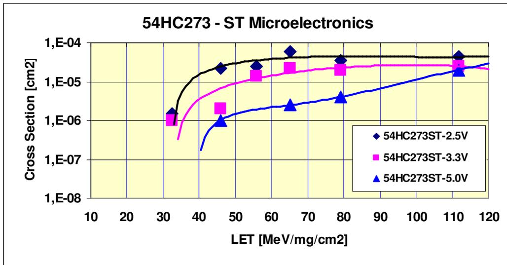
Figure 4.2.3 . Cross Section versus LET value for 54AC273 from ST Microelectronics. The graph shows the average results of two tested devices.
