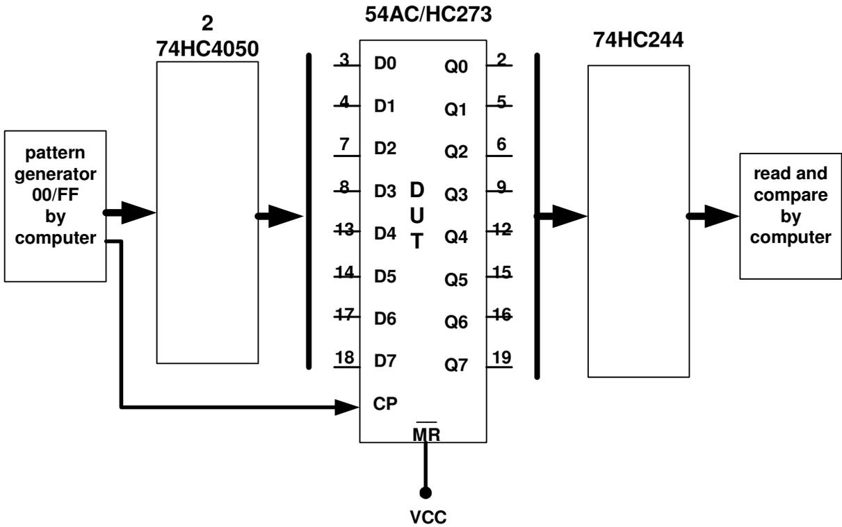
Fig 3.6.1 Test configuration diagram of 54AC273 / 54HC273. Logics at input and output are used for voltage adaption to the various test voltages of the DUT.
