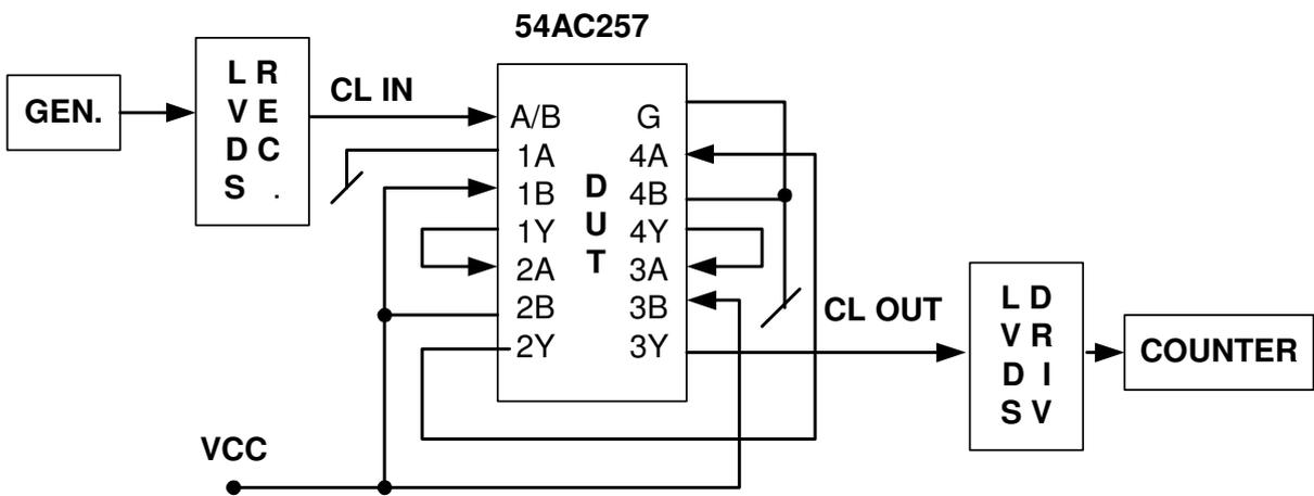
Fig 3.5.1 Test configuration diagram of 54AC257
