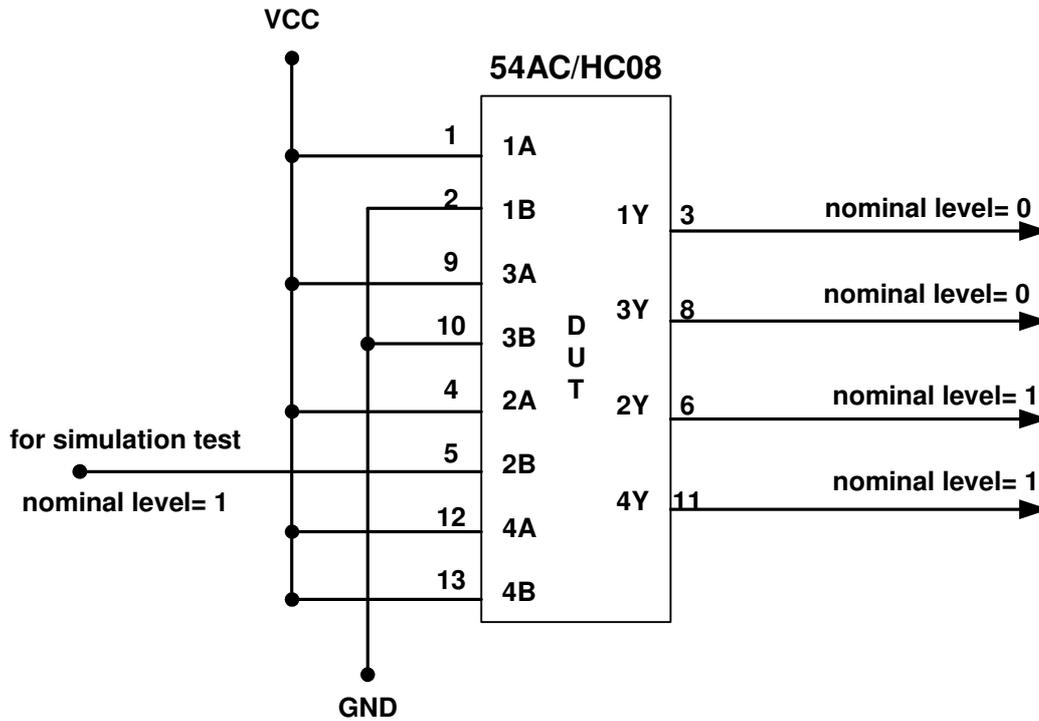
Fig 3.2.1 Test configuration diagram of 54AC08 / 54HC08
