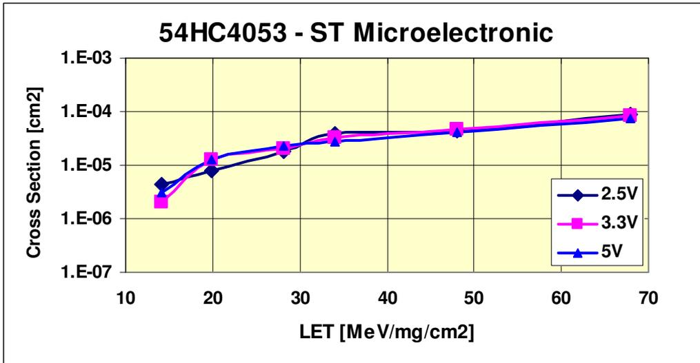
Figure 4.3.1 . Cross Section versus LET value for 54HC4053 from ST Microelectronics. The graph shows the average results of two tested devices.
