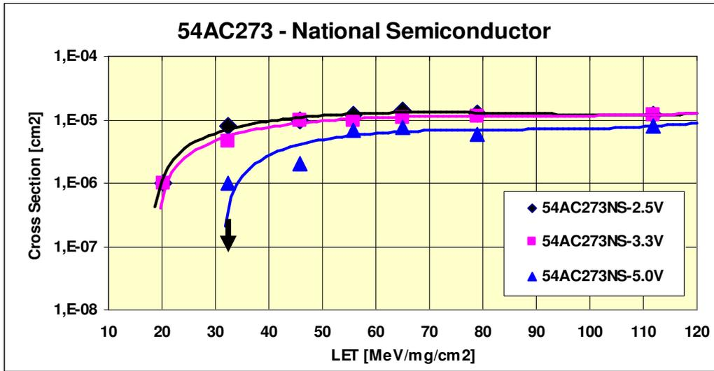
Figure 4.2.1 . Cross Section versus LET value for 54AC273 from National Semiconductor. The graph shows the average results of two tested devices. The arrow at 1E-7 MeV/mg/cm<sup>2</sup> indicates zero measured SEU.
