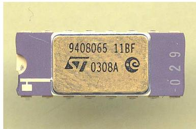
Fig 3.8.2 Picture of the top side of the package for 54HC4053 from STM
