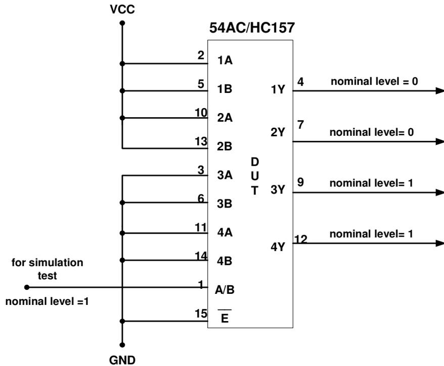
Fig 3.3.1 Test configuration diagram of 54AC157 / 54HC157
