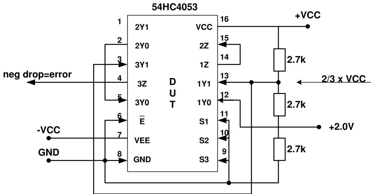
Fig 3.8.1 Test configuration diagram of 54HC4053
