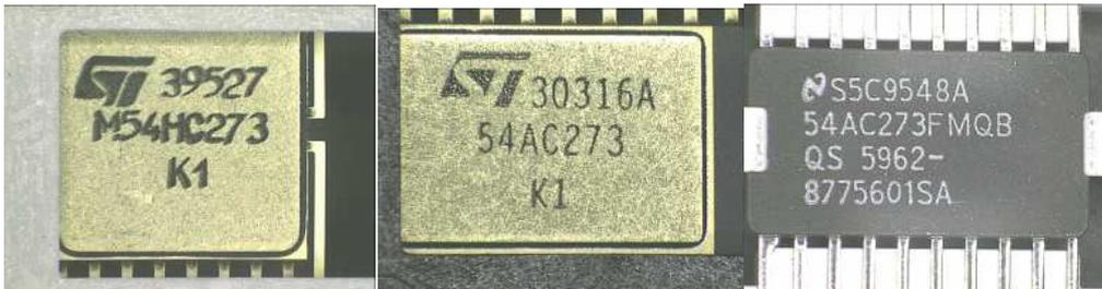
Fig 3.6.2 Picture of the top side of the packages for 54HC273 from STM. 54AC273 from STM and 54AC273 from NS
