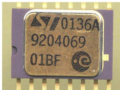
Fig 3.7.2 Picture of the top side of the package for 54HC4040 from STM
