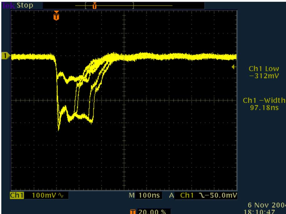
Figure 4.3.2 SET pulse shape for 54HC4053, LET=14 MeV/mg/cm<sup>2</sup>, Vcc=5V
