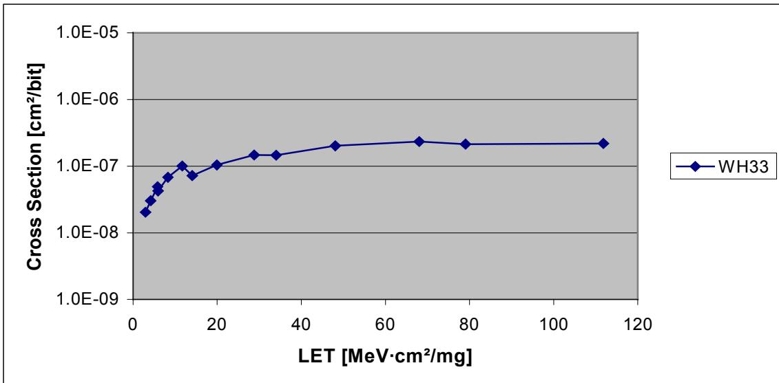
**Fig. 6: Cross section for WH33**
