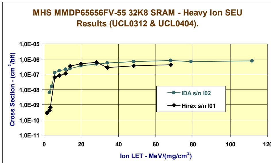
Fig. 8: Comparison of test results for MH51
