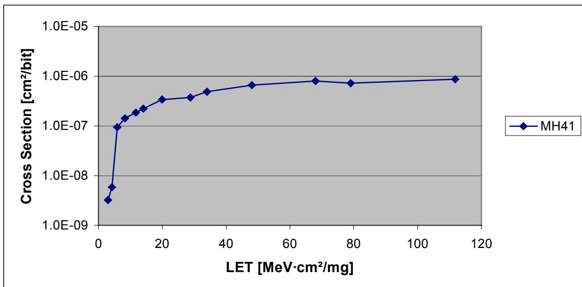
Fig. 4: Cross section for MH41
