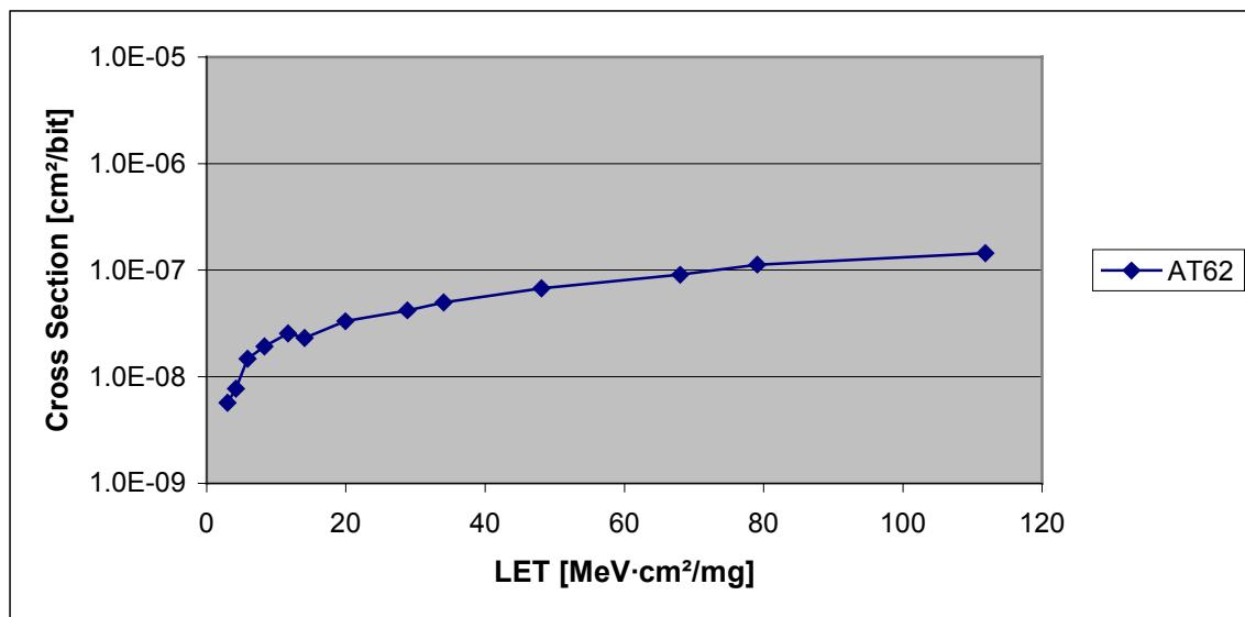
Fig. 3: Cross section for AT62
