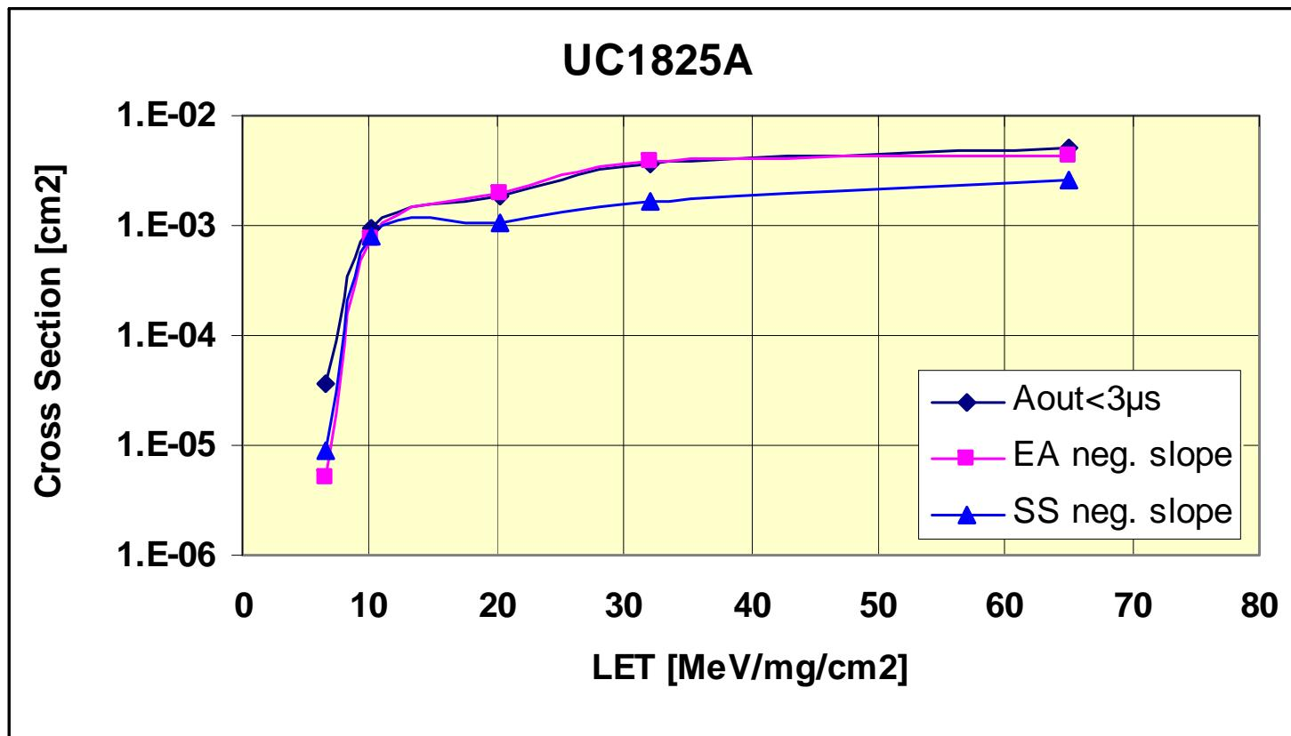
Trigg on Aout<3μs and EA negative slope show identical cross sections
