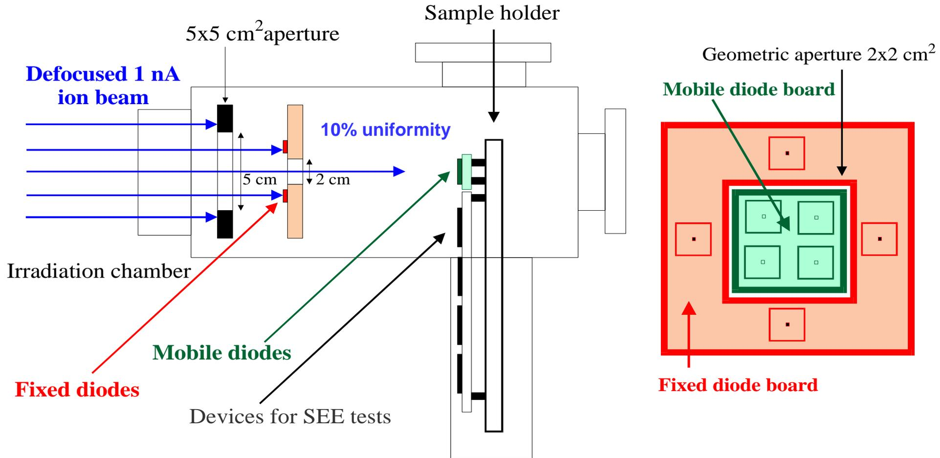
The **on-line beam monitoring system for defocused beams** by the fixed and mobile diodes:
