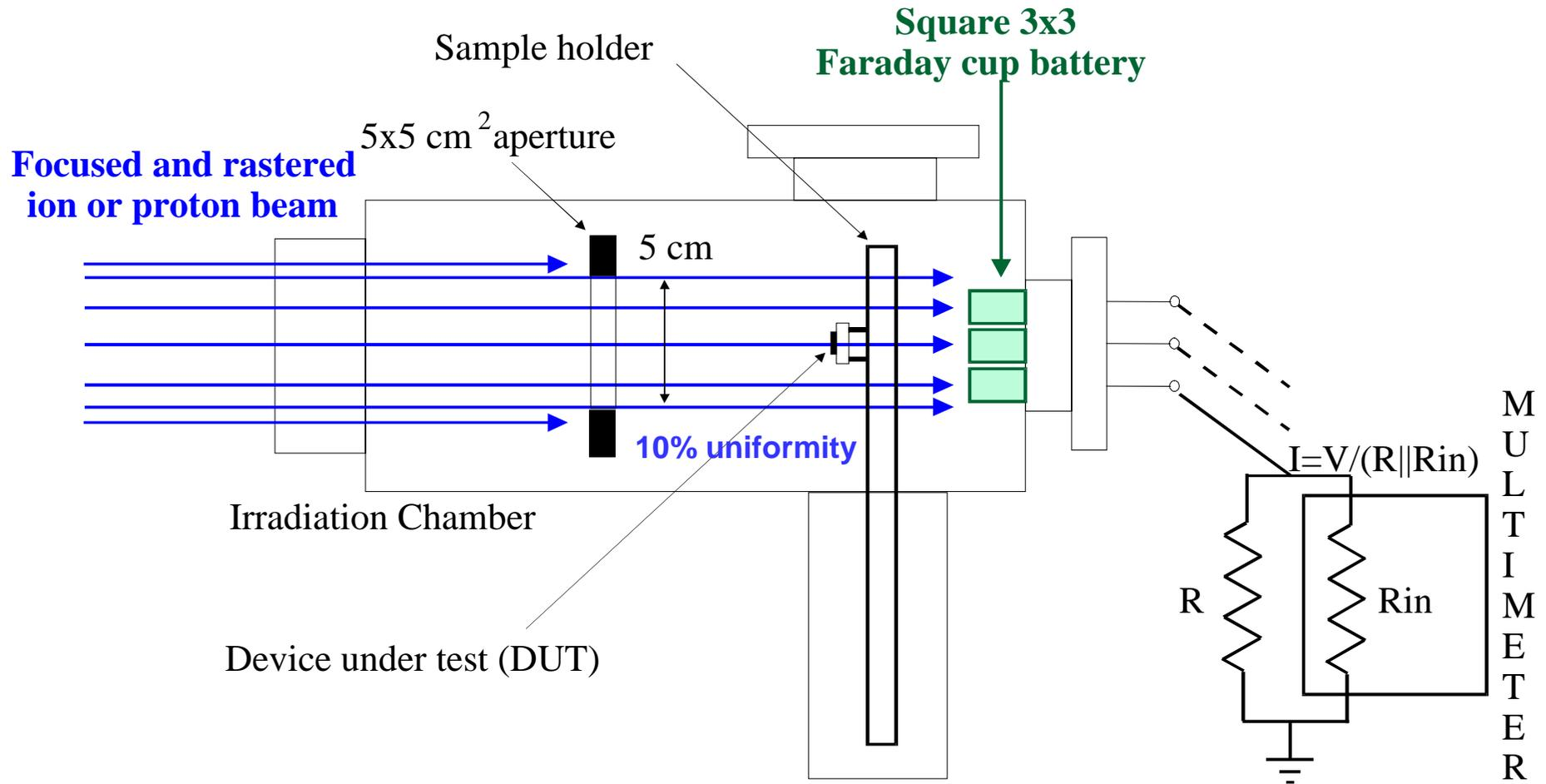
The **on-line beam monitoring for rastered proton and ion beams** by the 3×3 battery of Faraday cups positioned behind the DUT: side view of the experimental setup. The aperture of each Faraday cup is 0.6×0.6 cm<sup>2</sup>. The figure is not drawn to scale.
