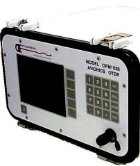
Optical Time Domain Reflectometer (OTDR)
