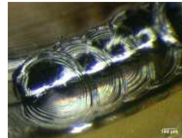
Solder joints for the output optical pigtail
