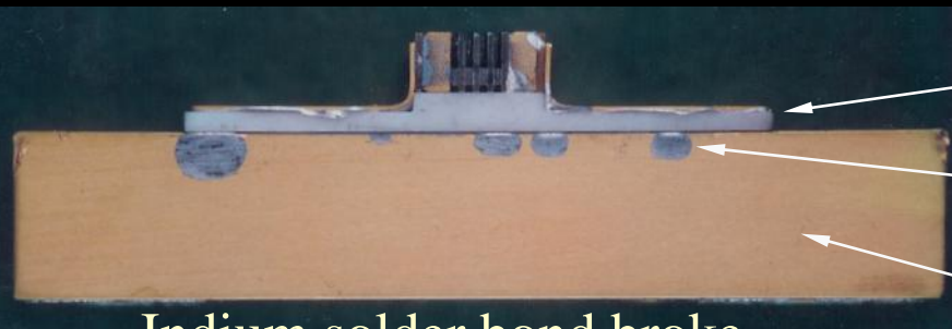
Indium solder bond broke
