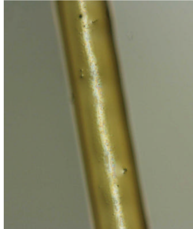
Typical “blistering” (inadequate cure between coats)
