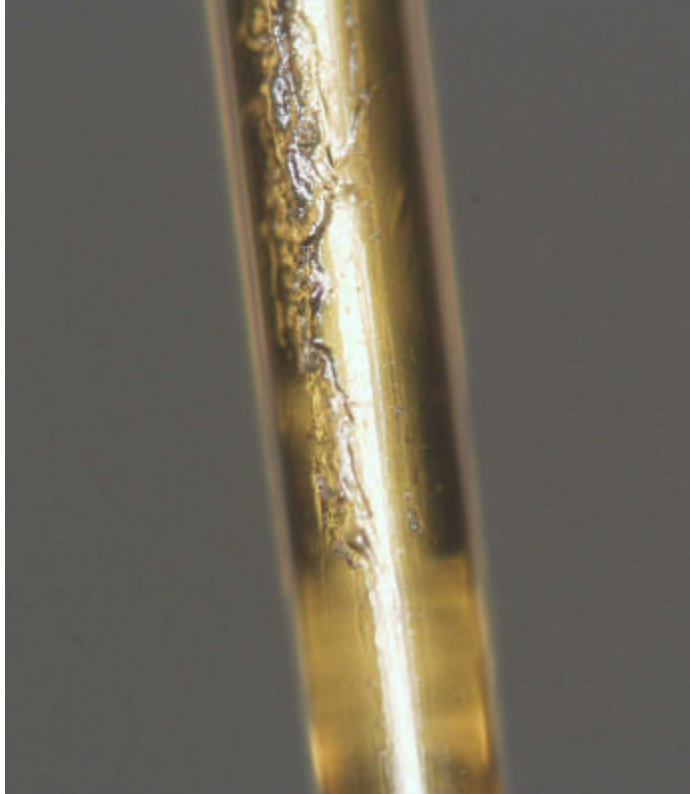
Typical “under curing” (post application reflow)
