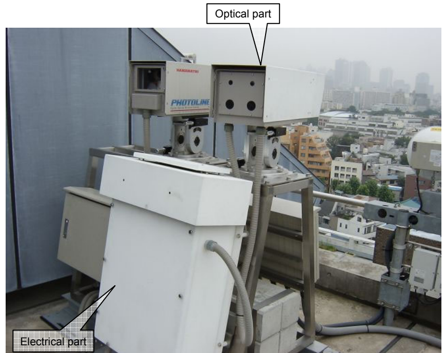
First fiber-to-fiber stable optical link was demonstrated in Waseda University campus at 1-km link distance.
