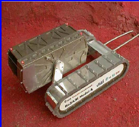
Nanokhod, ESA's future planetary rover (courtesy vH&S)
