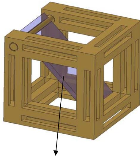
Wired-Grid Polarizer used as Polarizing Beam Splitter
