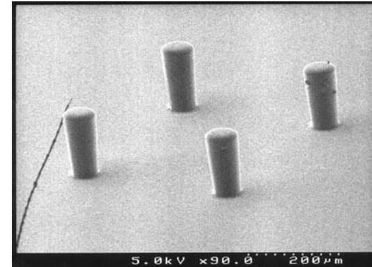
Flip-Chip VCSEL Using Compliant Polymer Bumps
