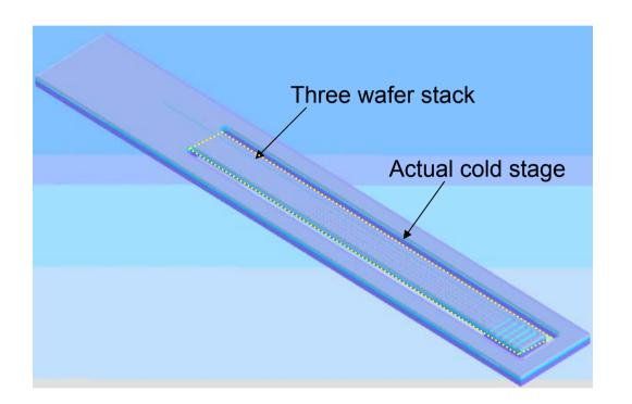
cold-stage length: 28 mm cold-stage width: 2.2 mm
