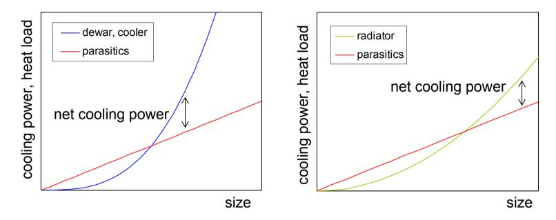
In cryocooler design the dependence of cooling power on size can be influenced regenerative cooler:  $\dot{Q}_L \sim f \times \Delta p \times V_{gas} \longrightarrow$  frequency *f* can be increased recuperative cooler:  $\dot{Q}_L = \dot{m} \times \Delta H_{gas}$   $\longrightarrow$  compressor design can be used with size-independent flow (e.g. sorption)
