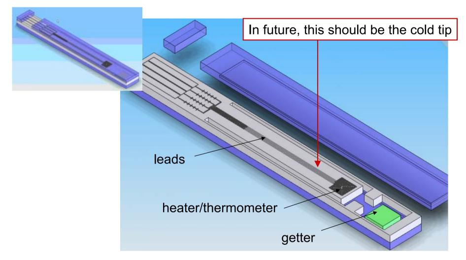
test chamber under construction: gas pressure to be monitored via thermal conductivity (Pirani-principle)
