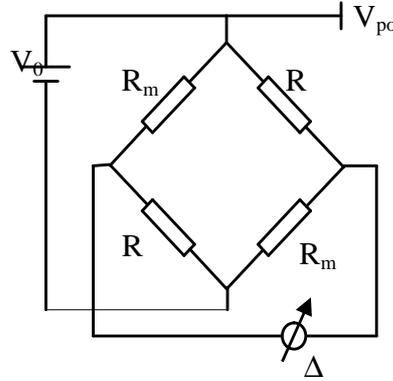
Fig.2 Wheatstone bridge resistor configuration
