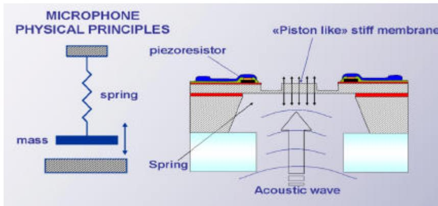
Fig.1 Device cross section.
