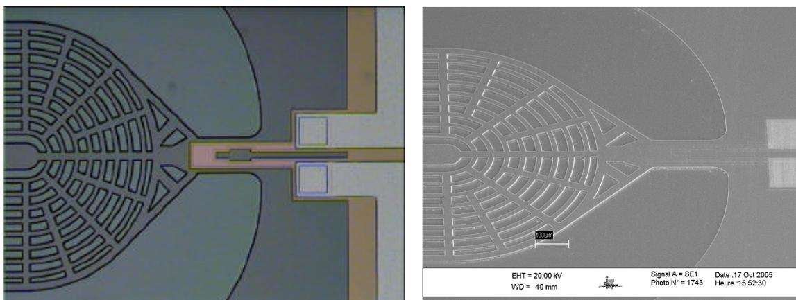
*Fig.5 Optical and SEM photographs of a piezoresistor on the cantilever structure after fabrication process.*
