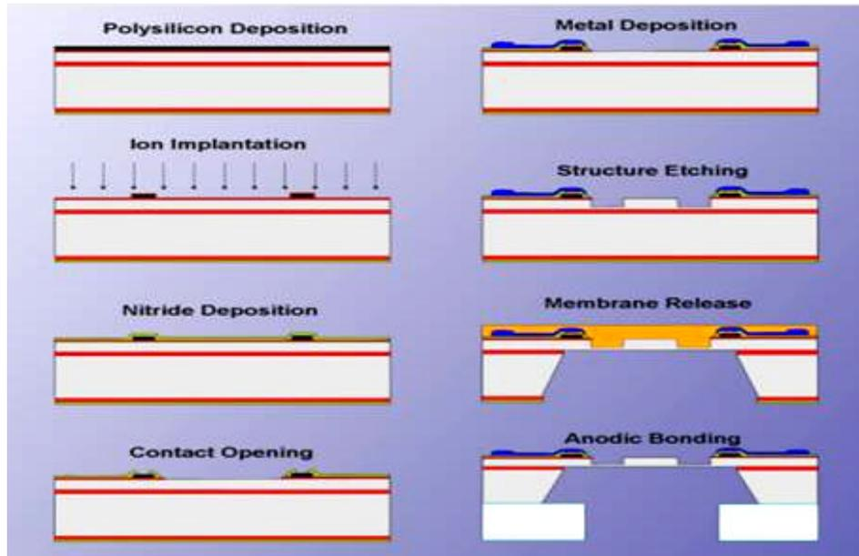
*Fig.4 Main fabrication process steps.*
