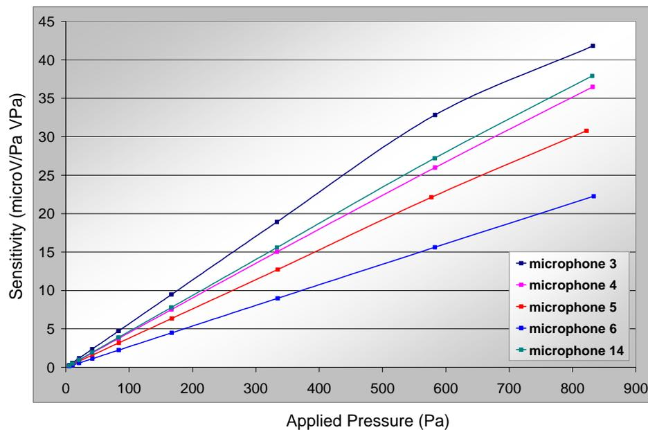
Fig.6 Measured potential as a function of applied pressure for different membrane thickness.
