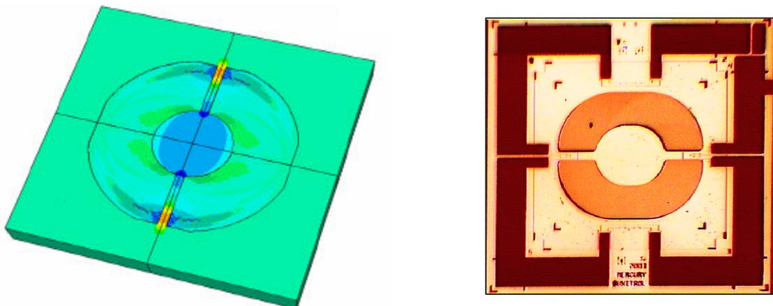
Fig.3 Simulation of the stress map by ANSYS (on the left) and design of the complete chip (on the right).
