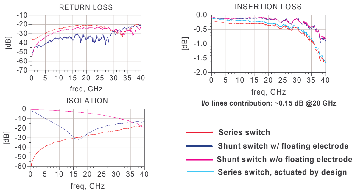
Fig. 5. Single switches RF-performance
