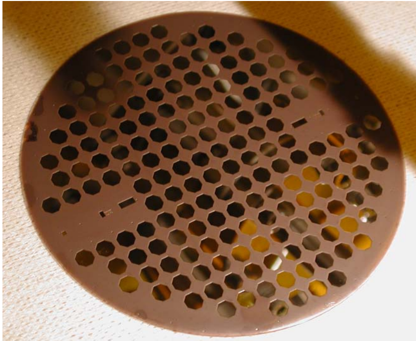
Chrome coated Pyrex7740 wafer with resist cavity mask defined
