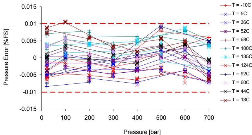
Fig. 2. Pressure error versus applied pressure at different temperatures.
