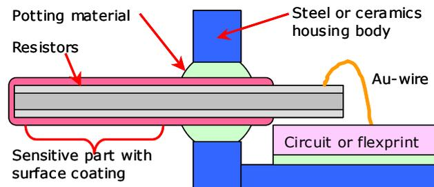
Fig. 5. Small diameter packaging concept.
