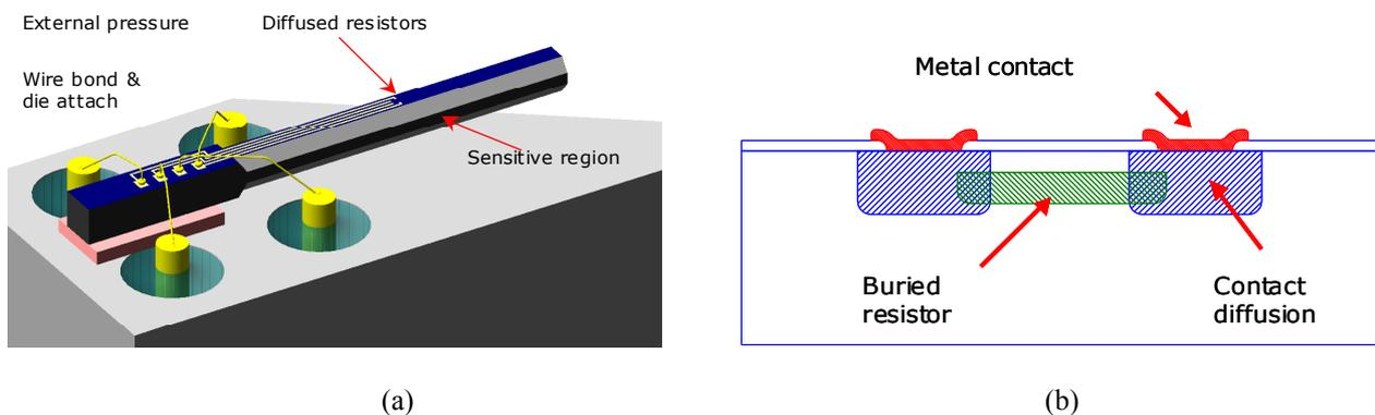
Fig. 1. Tubular silicon sensing element and assembly concept a), and diffused resistor bridge cross section b).
