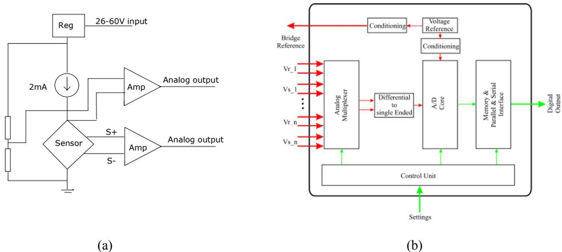
Fig. 7. Analog conditioning and interface circuit measurement set-up a) and digital interface ASIC block diagram b).
