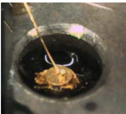
Compromised glass to metal seal
