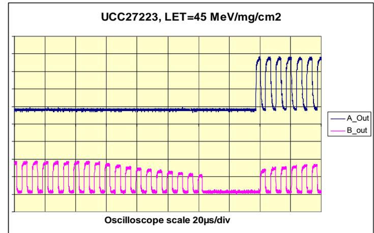
*Oscilloscope picture of output A and B showing worse case errors observed during irradiation with Kr-ions tilted at 45° (Let=45.4 MeV/mg/cm<sup>2</sup>).*
