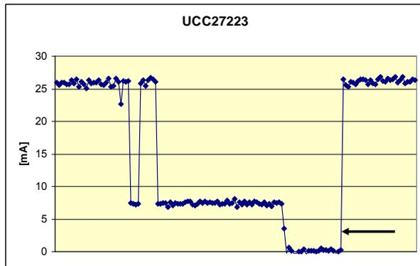
*Current jumps caused by irradiation. The arrow indicates where a reset has been performed by switching off - on the pulse generator to the input*
