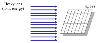
For each value of equivalent LET of the ion test, the cross section (where N<sub>SEE</sub> is the total number of SEE measured one run up to the fluence F).
