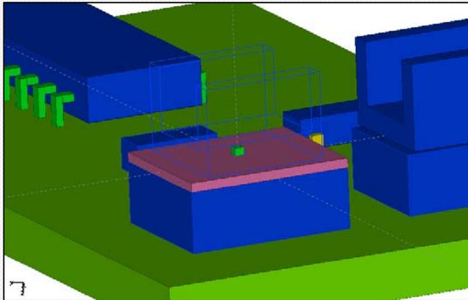
View of the OSL part : the « SFH425-D5 » detector is placed at the center of a Gallium-Arsenide die (in green) and the « OSL » detector at the center of the Strontium-Sulfide layer (in pink)
