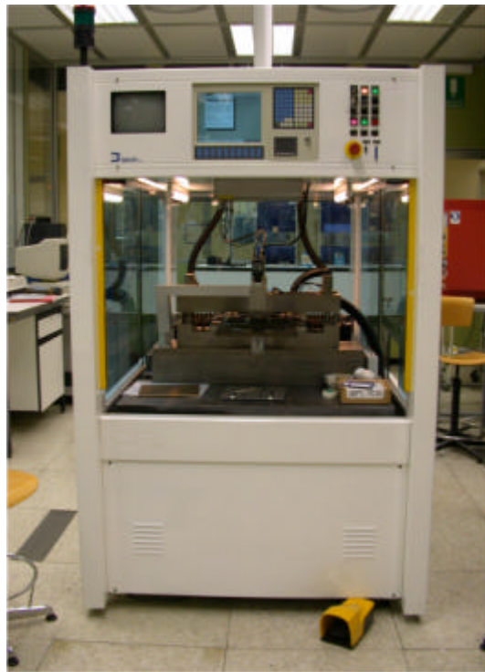
Puncher (10 holes /s), 100-150 \mu\text{m} diameter
