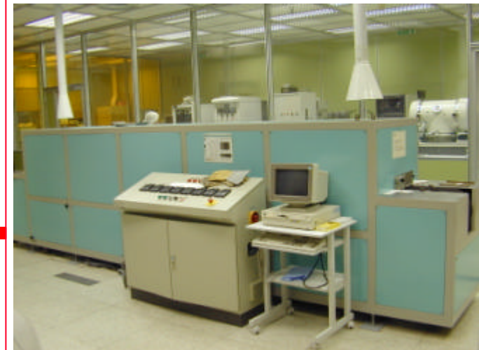
Firing belt oven ( T_{\max}=875^{\circ}\text{C} )
