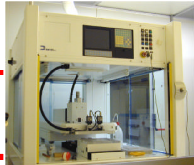
Screen Printing Machine - 100 \mu\text{m} lines
