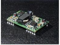
• Optimized thermal design, **buried thermal drain in the PCB**, heat dissipation possible by conduction through chassis mounting
