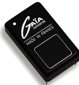
4W module DIL24 package, 7.5mm height
