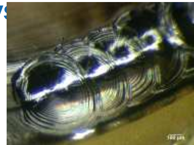
Solder joints for the output optical pigtail
