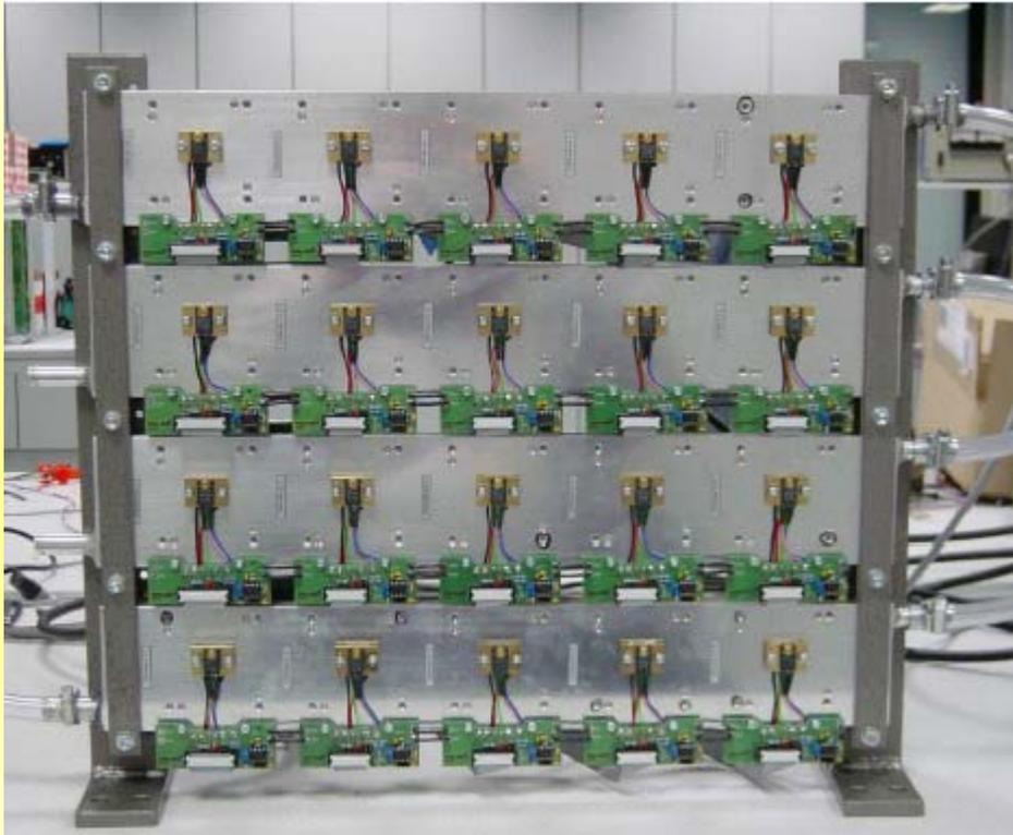
Endurance test bench setup under a class 100-1000 laminar flow box. Laser diode holder with protecting tube.
