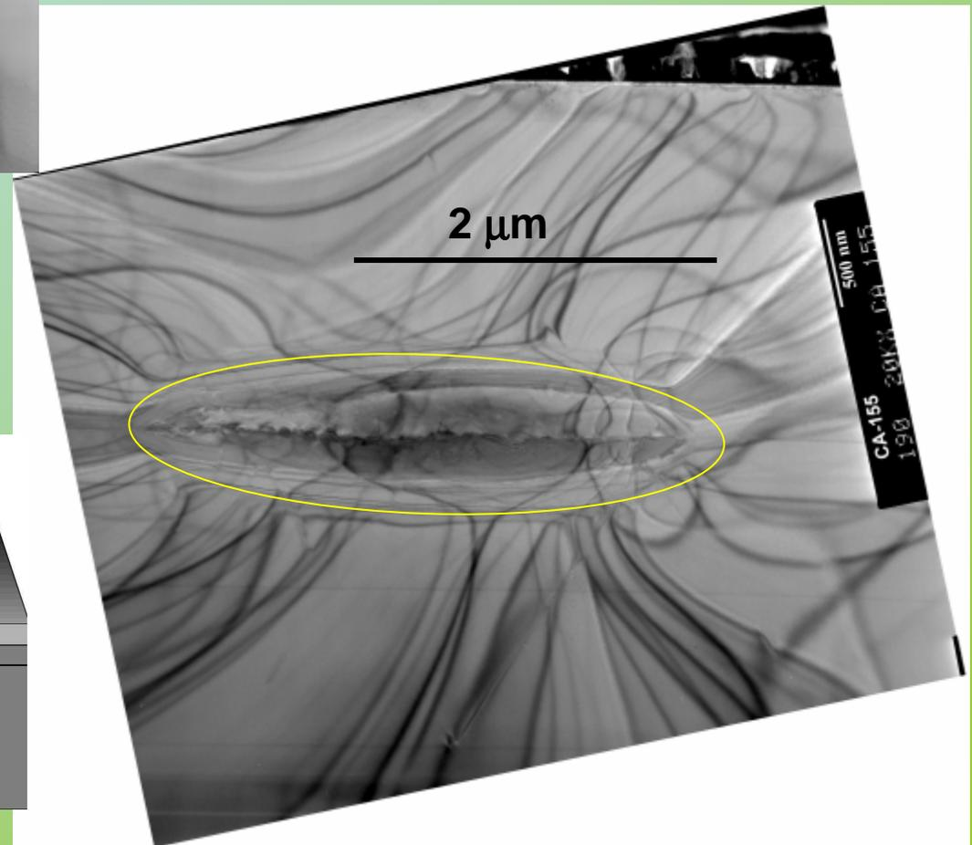
Fusion and re-crystallization, as for the "old" devices
