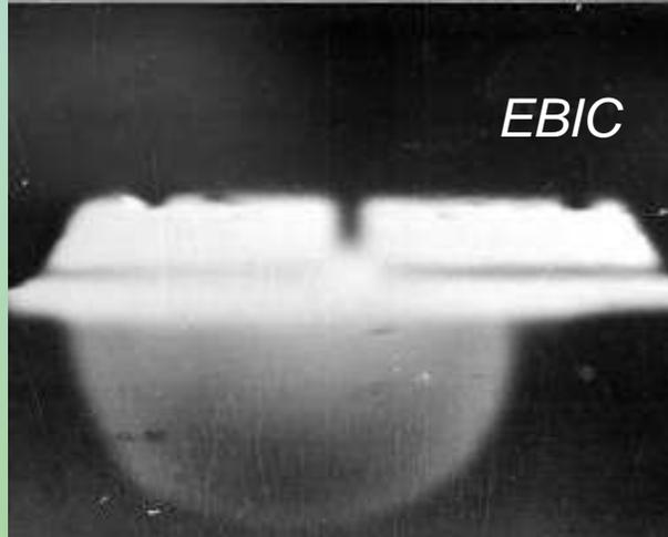
Degradation after THB tests.
