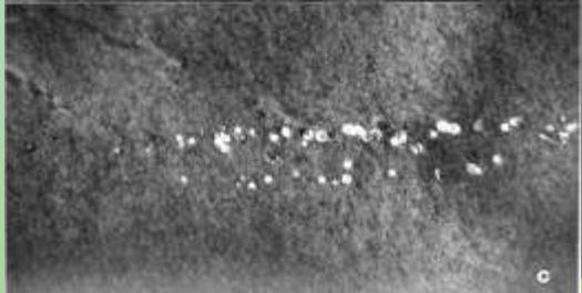
DLDs appeared as a network of dislocations and of dislocation loops, evolving from native defects at the epitaxial AlGaAs/GaAs interfaces under the effect of temperature (and recombination, as demonstrated years later)
