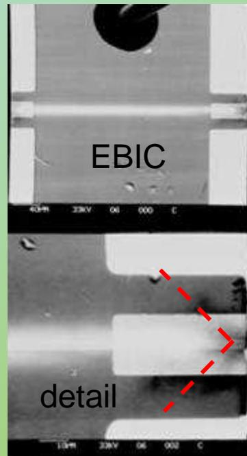
until EBIC started to reveal lattice-oriented dark stripes at the “burned” mirrors
