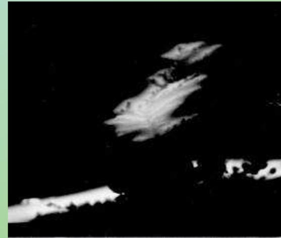
EBIC again: the discovery of a parasitic diode. Mechanism: corrosion
