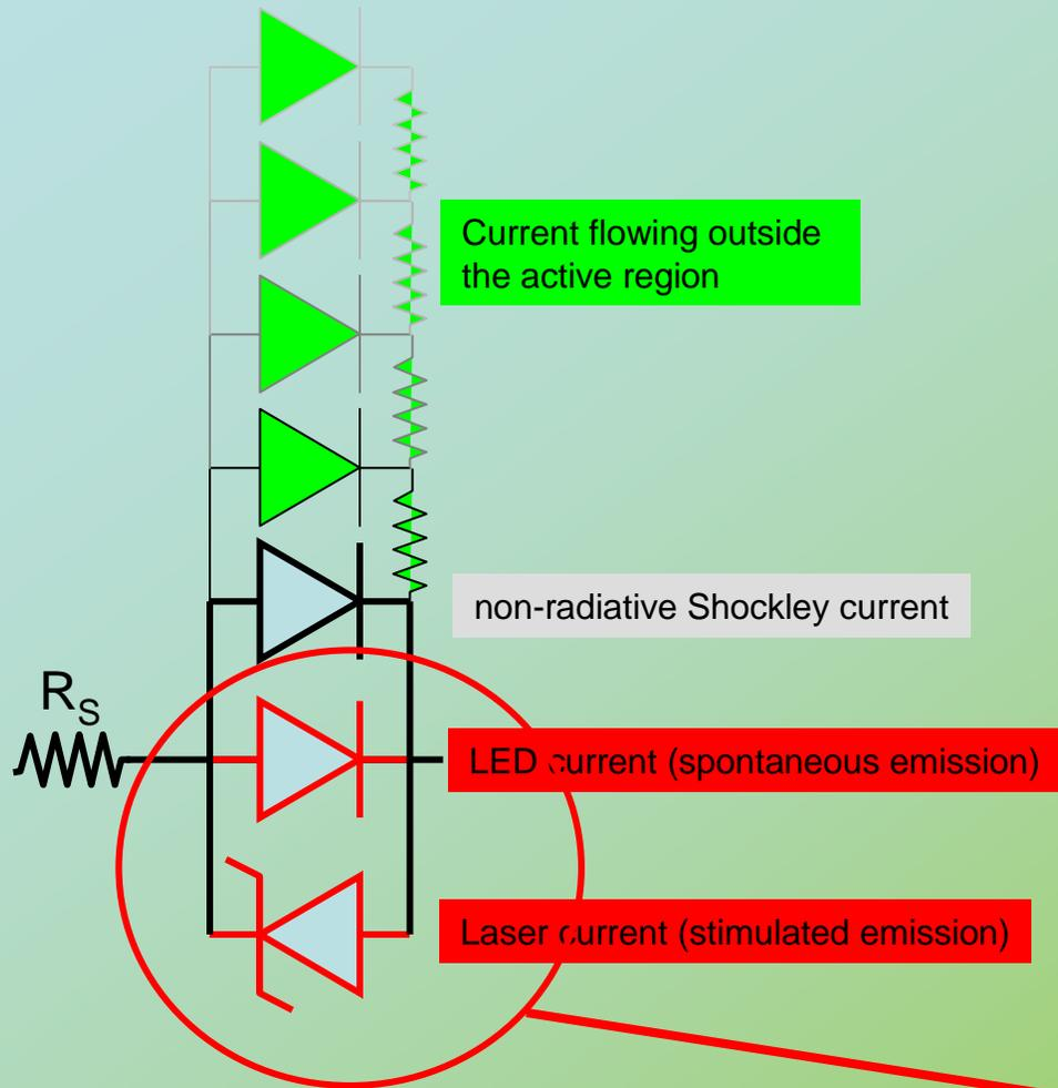
A multimodal (spectral) model linking  $I$ ,  $V$  and the spectral power.
