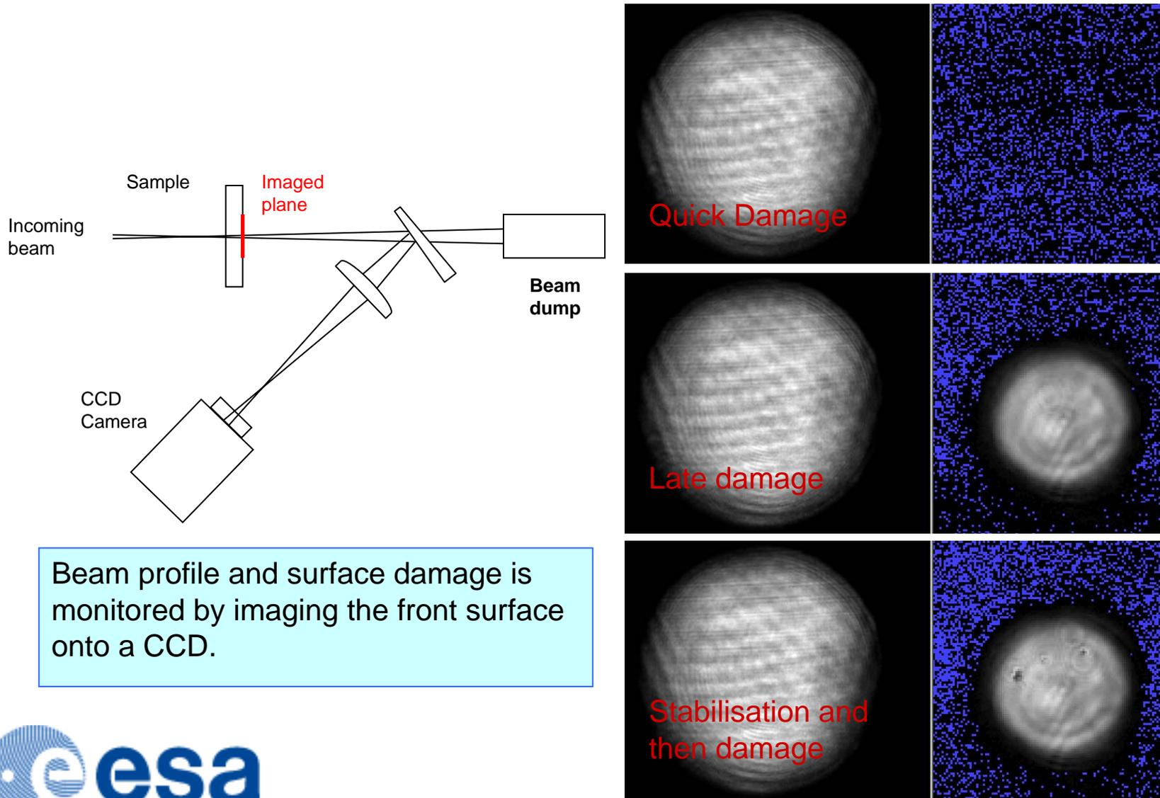
Beam profile and surface damage is monitored by imaging the front surface onto a CCD.
