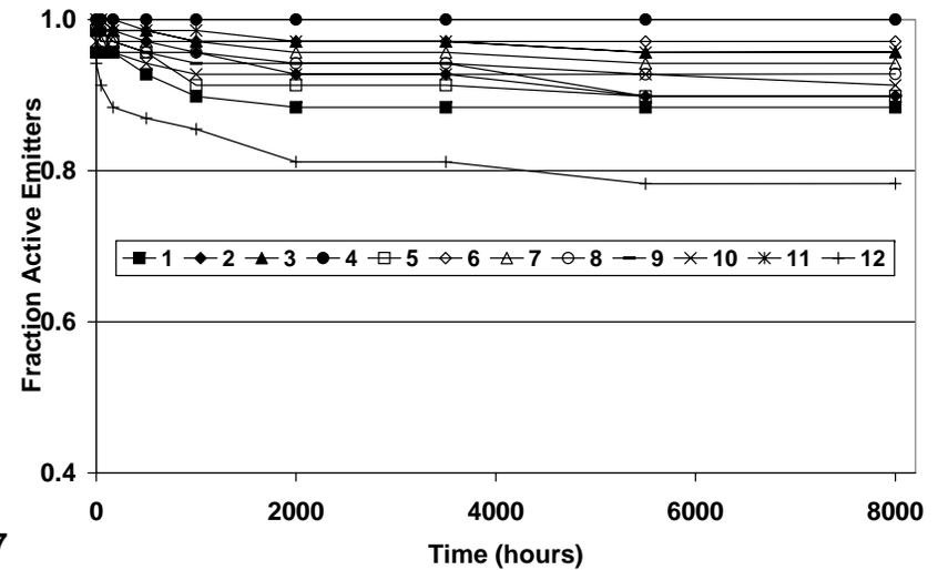
Evolution of the fraction of active emitter within one stack
