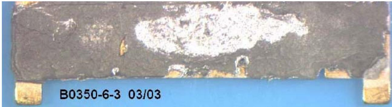
Solder between heat sink and Cu mount: intermetallic compound
