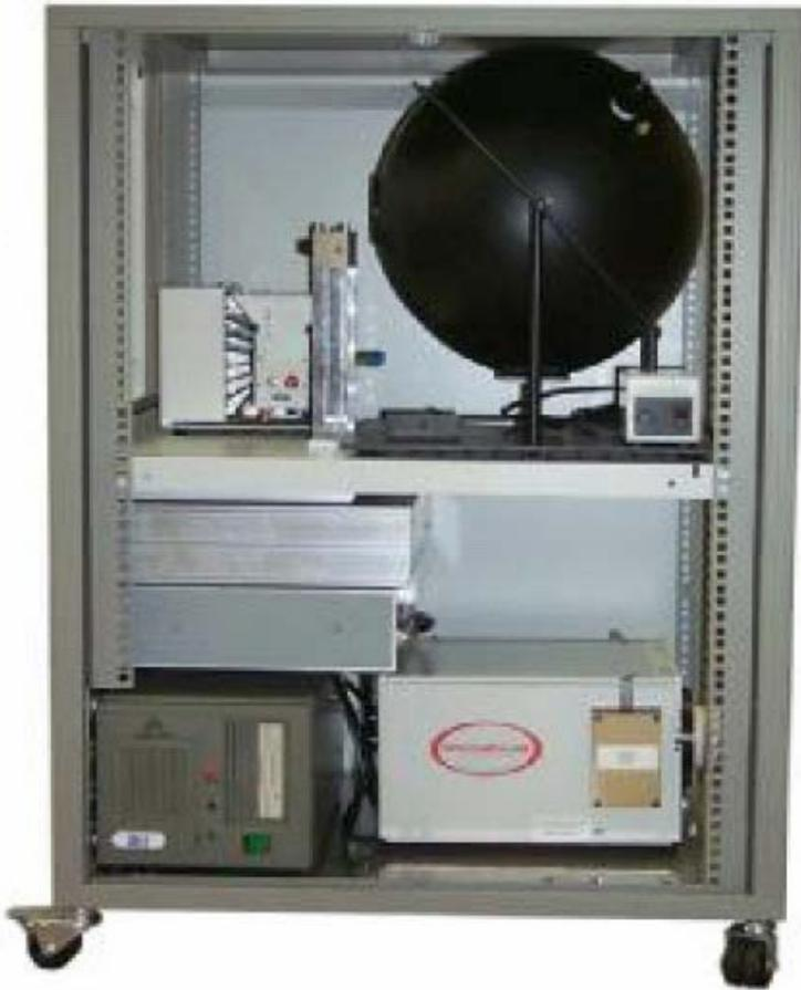
**Mobile electro-optical characterisation setup**
