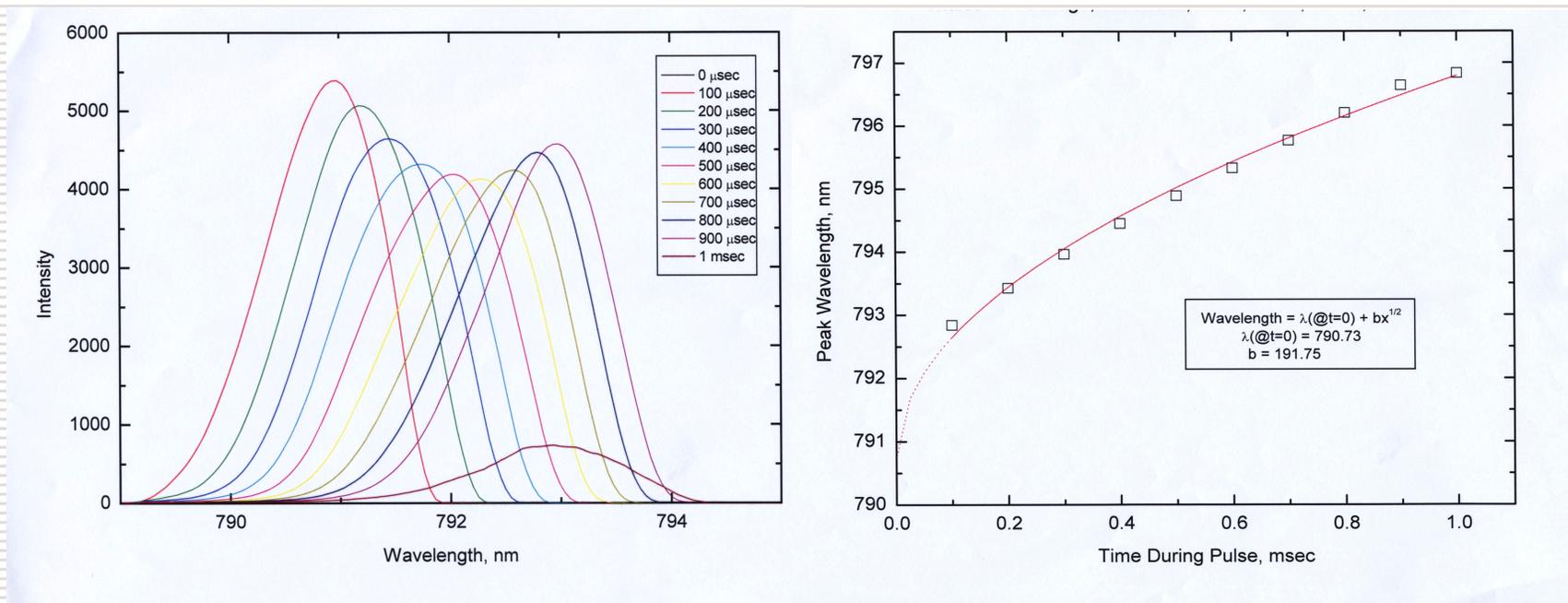
Spectral Shift during Pulse = 6 nm
