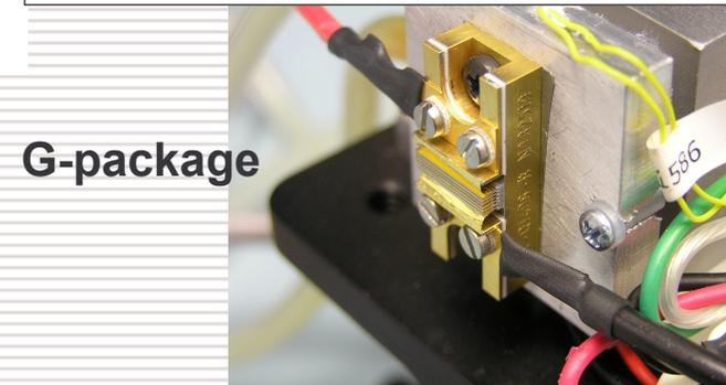
G-package bars run from 6 to 13 degrees cooler than A-package
