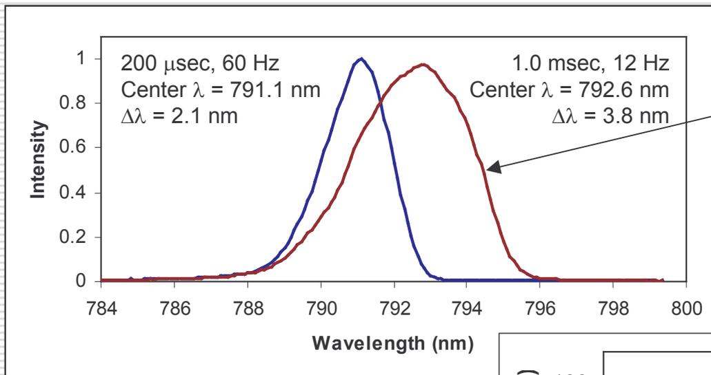
Spectral shift and broadening due to thermal cycling
