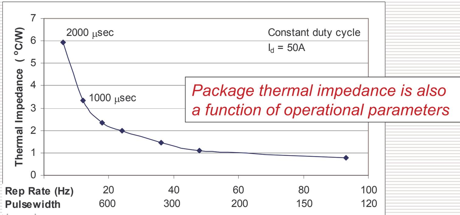
Varying pulsewidth (125 μsec to 2 msec) and repetition rate while keeping duty cycle constant at 1.2%
