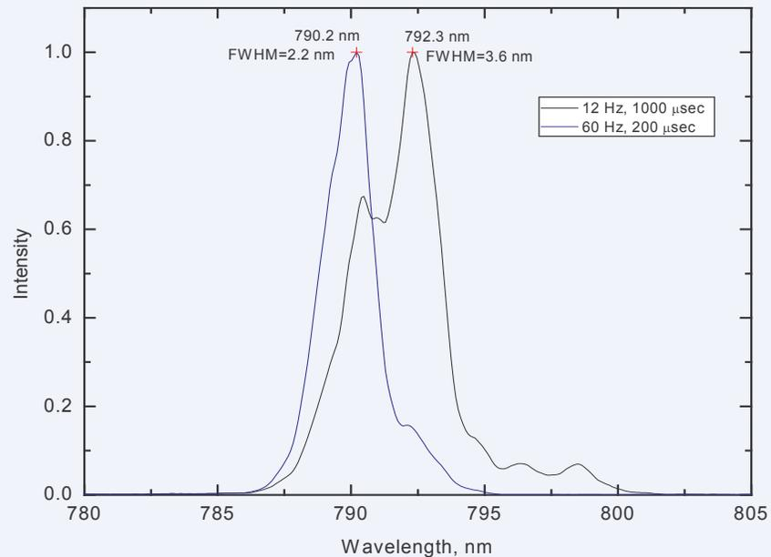
Spectral response at 200  $\mu$ sec and 1 msec pulse durations
