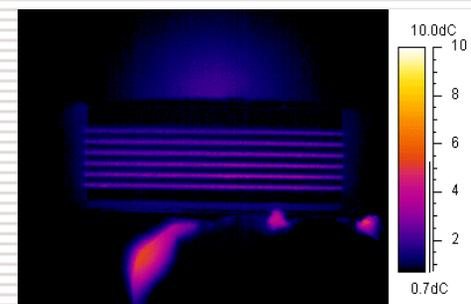
A-6 Array with some failing emitters (15% drop in power)
