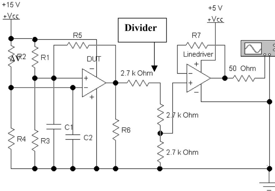
Fig. 1 Schematic drawing of the comparator test setup. The resistance dividers R1/R2 and R3/R4 maintain input voltage differences. The box to the right represents the oscilloscope with 50  $\Omega$  input resistance. R1 = 26.1 k $\Omega$  or 5.72 k $\Omega$ , R2 = 26.1 k $\Omega$ , R3 = 5.62 k $\Omega$ , R4 = 5.23 k $\Omega$ , R5 = 562 k $\Omega$ ,
