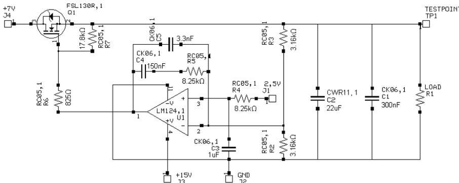
Fig. 2 Schematic drawing of the 5-volt regulator setup. The "load R1" is 115 $\Omega$ .
