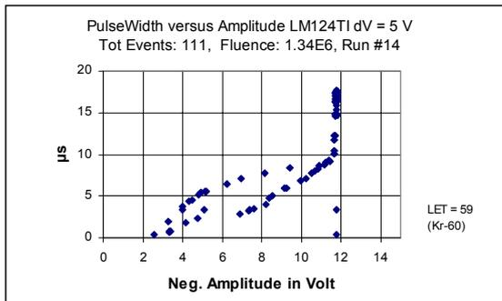
Fig. 11 Scatter diagram showing the pulse length at FWHM vs. the amplitude,  $\Delta V_{in} = 5V$ .
