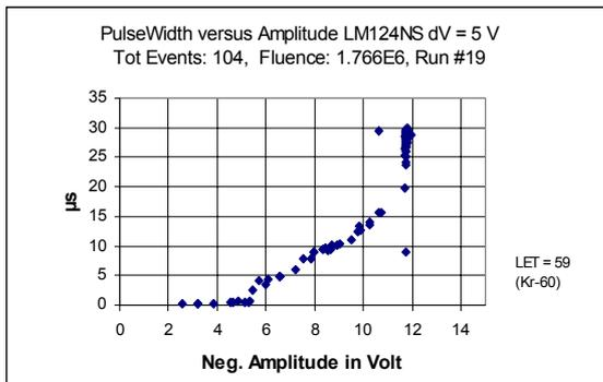
Fig. 5 Scatter diagram showing the pulse length at FWHM vs. the amplitude,  $\Delta V_{in} = 5V$ .
