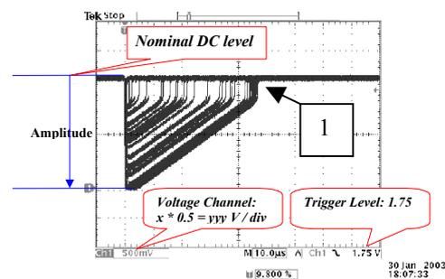
Fig. 3 Definition of the SET pulse amplitude
