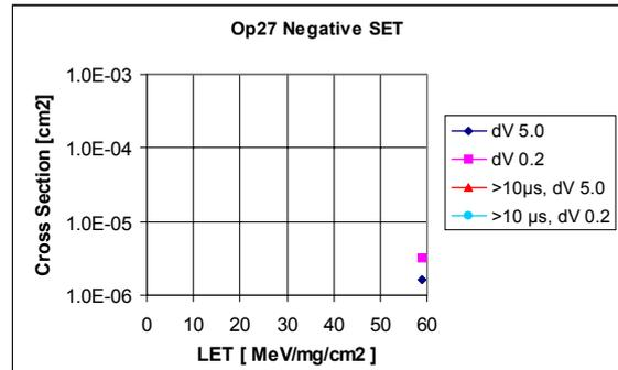
Fig. 13 SET cross-section vs. LET-value for all SETs and for the SETs longer than 10  $\mu\text{s}$  are given for delta input voltage respectively.
