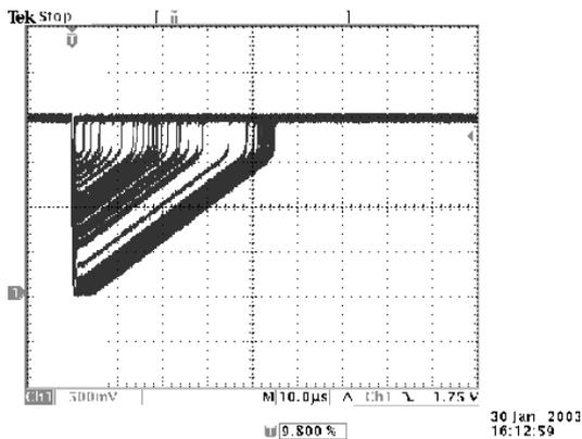
Fig. 6 Oscilloscope image of the SET's given in figure 2. X-scale = 10  $\mu\text{s}/\text{div}$ . (LM124NS)
