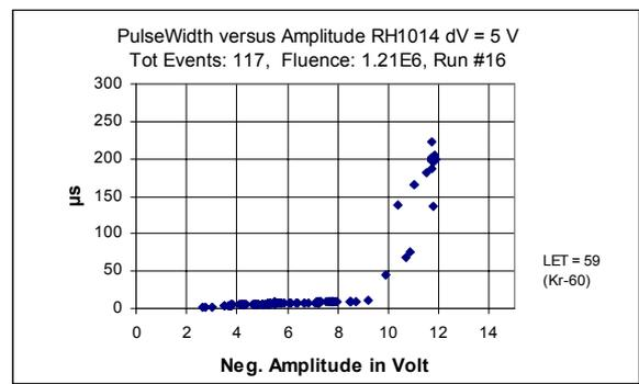
Fig. 8 Scatter diagram showing the pulse length at FWHM vs. the amplitude,  $\Delta V_{in} = 5V$ .
