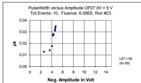
Fig. 14 Scatter diagram showing the pulse length at FWHM vs. the amplitude,  $\Delta V_{in} = 5V$ .
