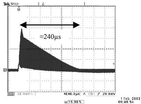
Fig. 17 Oscilloscope picture showing the positive going SET pulses.
