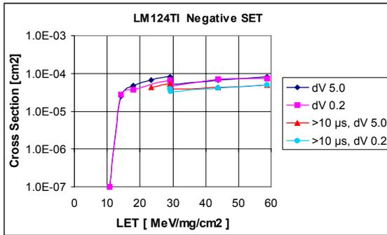
Fig. 10 SET cross-section vs. LET-value for all SETs and for the SETs longer than 10  $\mu\text{s}$  are given for delta input voltages respectively.
