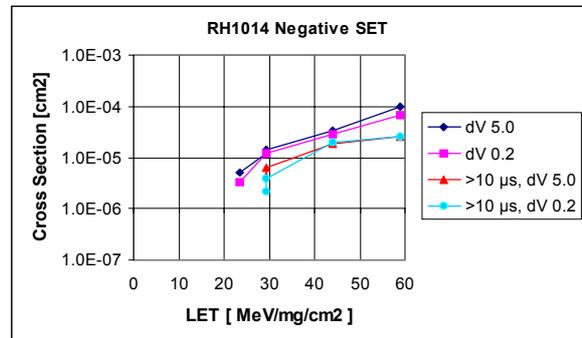
Fig. 7 SET cross-section vs. LET-value for all SETs and for the SETs longer than 10  $\mu\text{s}$  are given for delta input voltages respectively.
