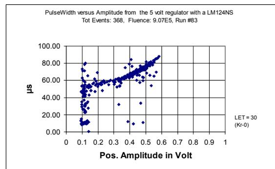
Fig 18 Scatter diagram showing positive pulse length at FWHF in  $\mu$ s vs. amplitude in Volt,
