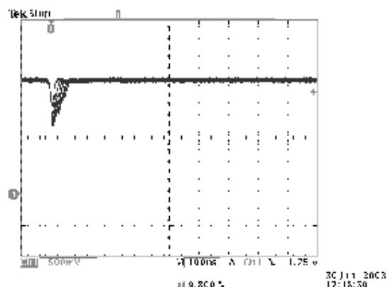
Fig. 15 Oscilloscope image of the SET's given in figure 11. X-scale = 100 ns/div. (OP27)
