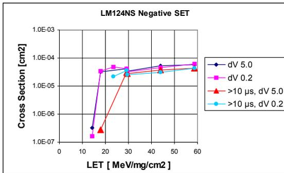
Fig. 4 SET cross-section vs. LET-value for all SETs and for the SETs longer than 10  $\mu\text{s}$  are given for delta input voltages respectively.
