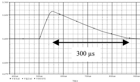
Fig. 19 Result from a PSpice simulation of the 5-Volt regulator.
