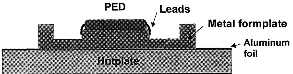
FIGURE IV – PRINCIPLE SET-UP FOR AUTOMATED WET ETCHING
