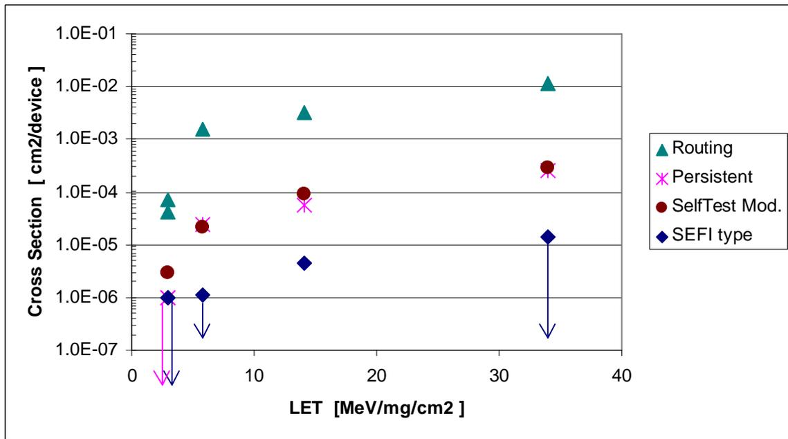
Figure 8.1 Configuration errors for non-TMR Design. Arrows indicate test without any upsets. The Cross sections are per device and are specific for this design. To predict cross section for a 100% utilised device you must multiply these cross sections (except SEFI type) with the utilisation factor for this design (about 32% for the routing and persistent errors and maybe 5% for the SelfTest module).
