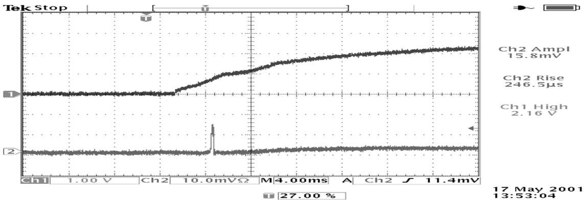
Figure 7.4 Oscilloscope image of  $V_{CCINT}$  (Ch1- 1V / div) and  $I_{CCINT}$  (Ch2- 0.2A / div) for the reference device, REF#33 (4ms / div). The current peak observed during the ramp-up of the voltage is according to specification [3].
