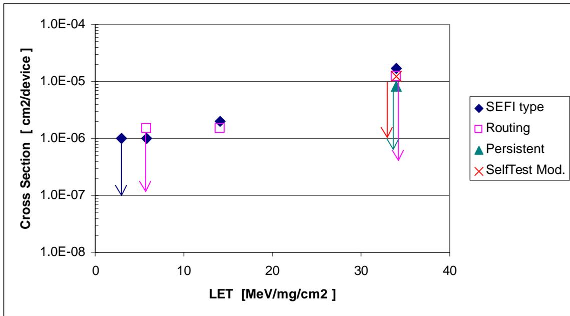
Figure 8.3 Configuration errors for TMR Design. Arrows indicate test without any upsets.
