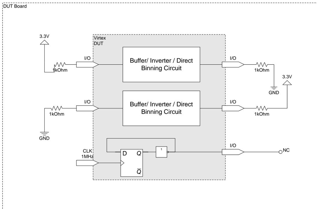
Figure 5.1 Principal drawing for configuration of I/Os during irradiation.
