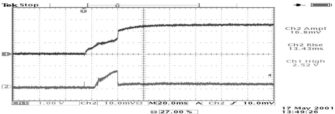
Figure 7.8 Oscilloscope image of  $V_{CCINT}$  (Ch1- 1V / div) and  $I_{CCINT}$  (Ch2- 0.5A / div) for sn#39 after 50krad(Si) (20ms / div). The current peak observed in the pre-irradiation case is here followed by further increase in the current until the voltage has reached 1.2V.
