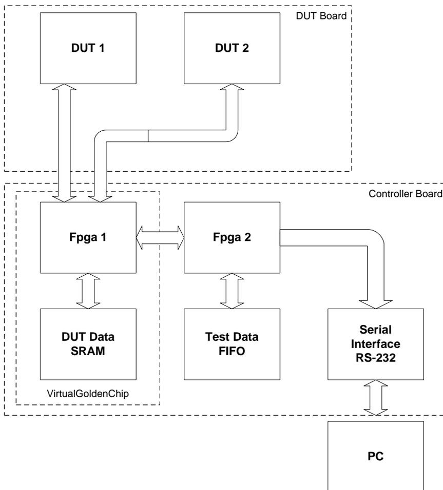
Figure 4.2 Principal drawing of DUT board and Controller Board
