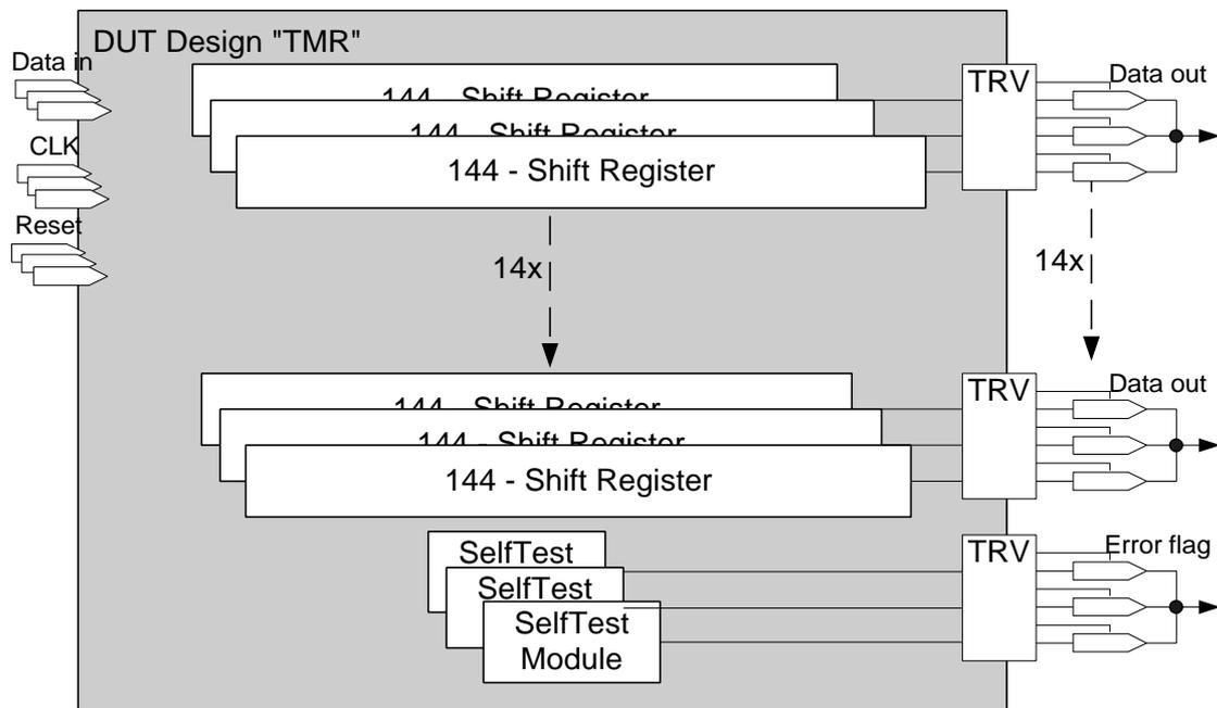
Figure 3.4 Principal Drawing of TMR DUT Design
