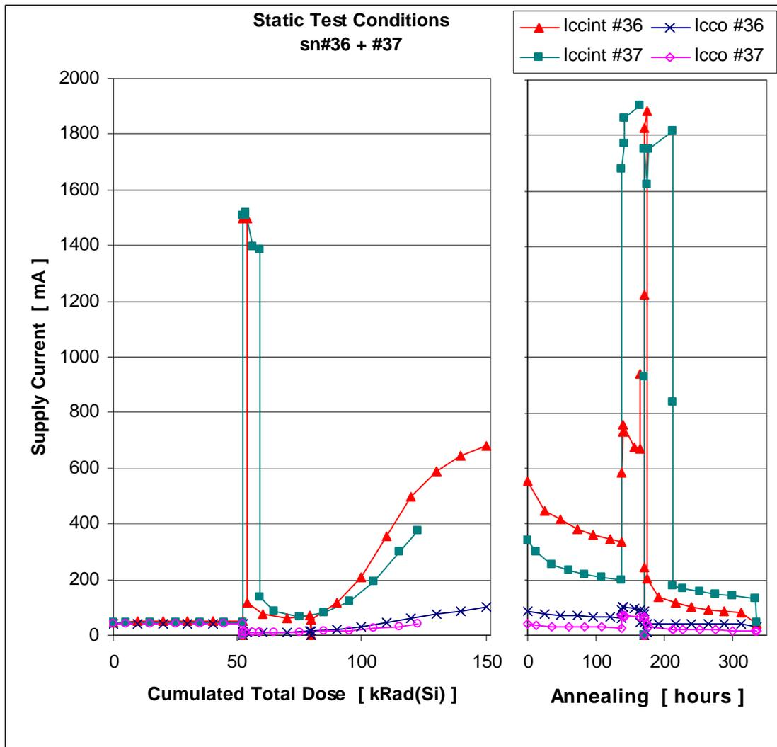
Figure 7.3 Supply current values during irradiation and annealing for sn#36 and sn#37 that was irradiated in static test conditions. After 50 krad(Si) both DUTs failed to initialise. The supply current for the I/O logic was just 10mA which indicates that the DUT wasn't configured. Sn#37 was removed between the 50 krad(Si) and 78krad(Si) irradiation step and therefor only received a cumulated total dose of 122 krad(Si).
