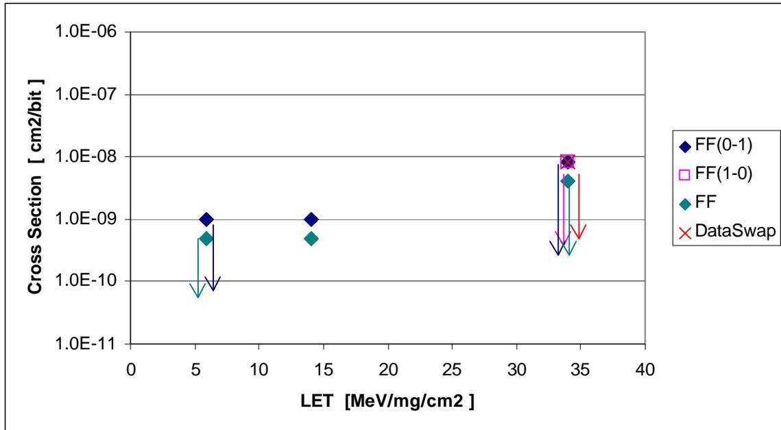
Figure 8.4 Register Errors of TMR Design. Arrows indicate test without any upsets.
