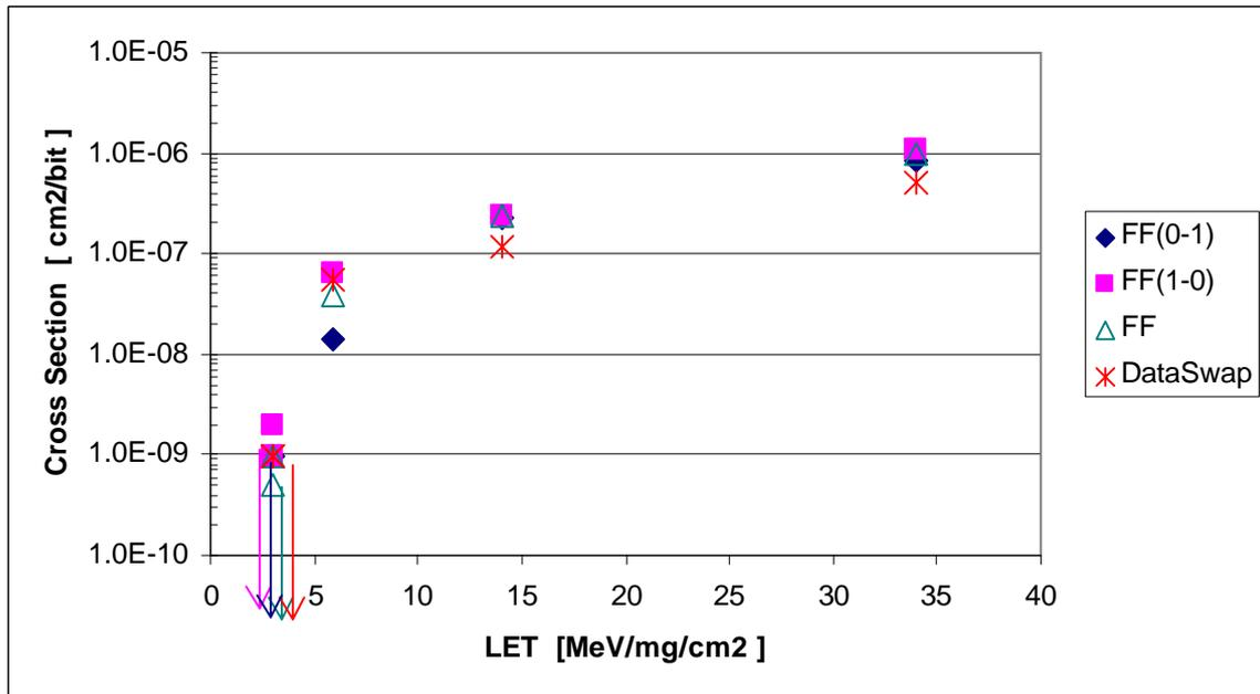
Figure 8.2 Register Errors for non-TMR Design. Arrows indicate test without any upsets.
