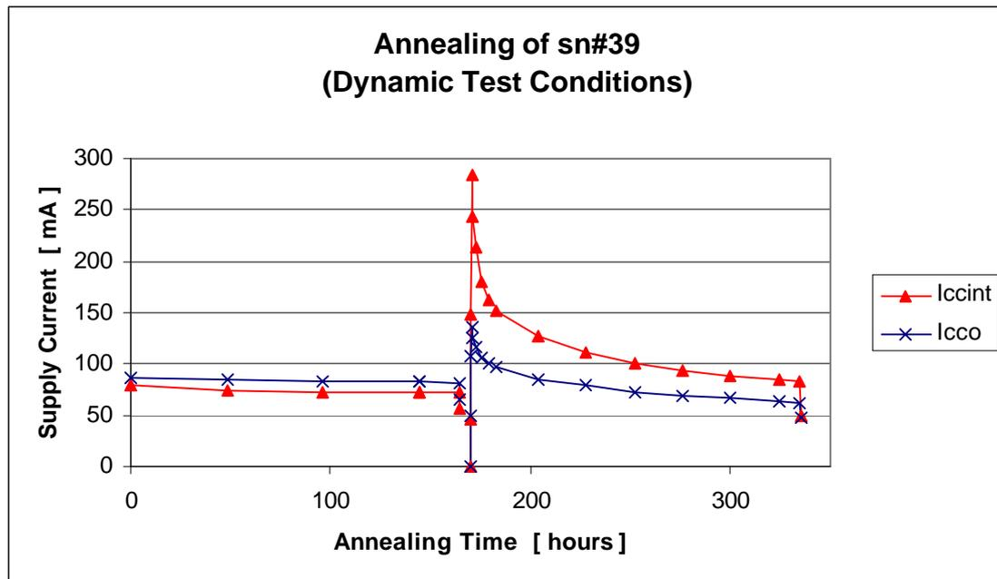
Figure 7.2 Supply current values for sn#39 during 168h room temperature and 168h 100 degree annealing. The device was static biased during annealing and not power cycled. After high temperature annealing the last measuring point is performed at room temperature. It can be seen that both currents decreased to less than 50 mA which were the pre-irradiation values. The high temperature annealing indicate a special anneal effect on the induced radiation damages.
