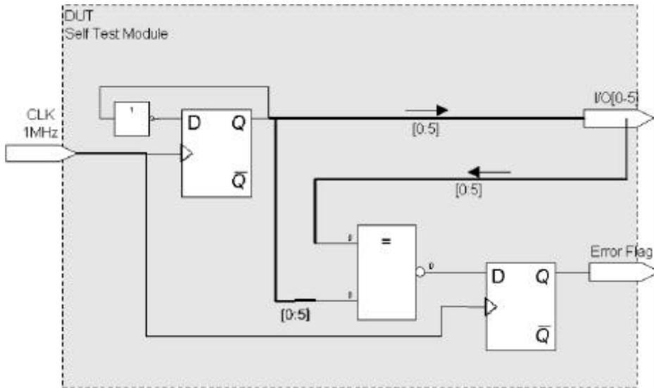
Figure 3.3 Principal Drawing of SelfTest Module
