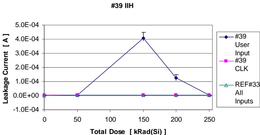
Figure 7.11 Average Input Leakage high Current for sn#39 for user I/Os and dedicated Clock. Measurement at 200 and 250 krad(Si) are the two annealing steps. All measurement over  $1.2 \times 10^{-4}$  A was made with another instrument. Error bars indicate max and min measured value for each device.
