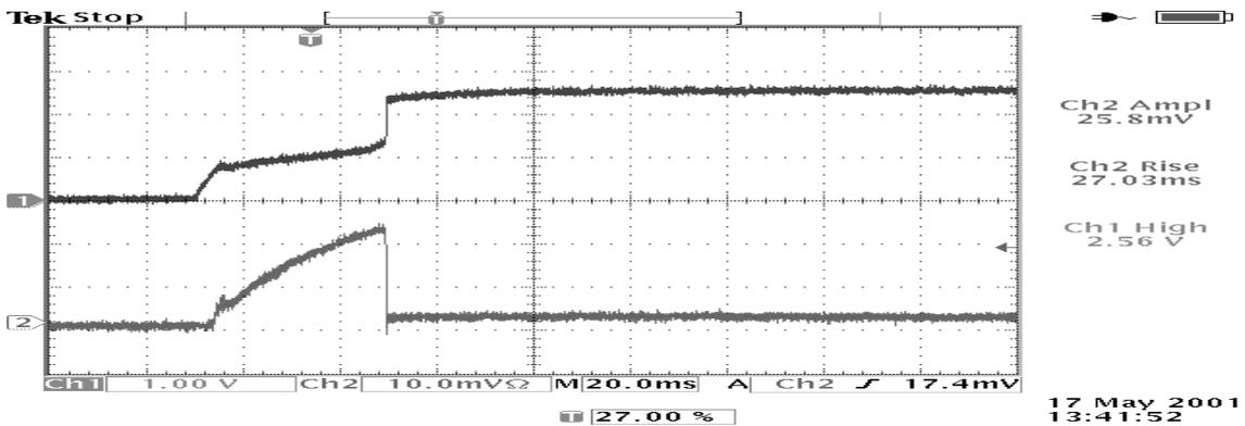
Figure 7.7 Oscilloscope image of  $V_{CCINT}$  (Ch1- 1V / div) and  $I_{CCINT}$  (Ch2- 0.5A / div) for sn#38 after 50krad(Si) (20ms / div). The current peak observed in the pre-irradiation case is here followed by further increase in the current until the voltage has reached 1.2V.
