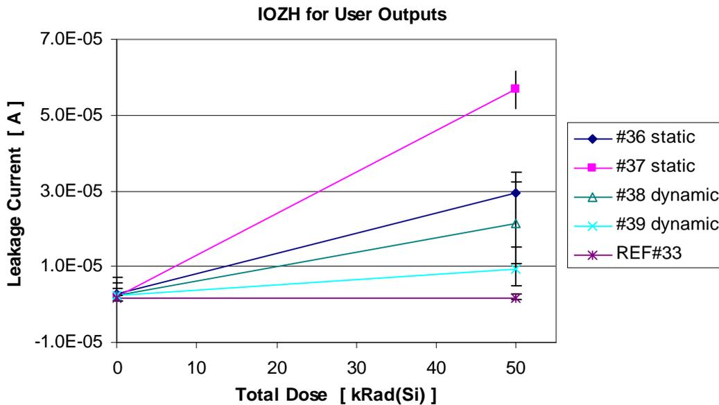
Figure 7.10 Average Output Leakage High Current for user I/Os and devices up to 50krad(Si). User outputs that were driven high during irradiation have been excluded. They had lower leakage than the outputs presented in this graph. Specification limit is  $1 \times 10^{-5}$  A. Error bars indicate max and min-measured value for each device.
