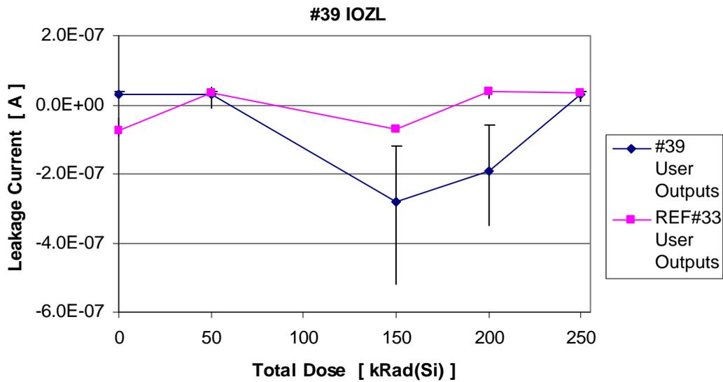
Figure 7.14 Average Output Leakage Low Current for sn#39 for user I/Os and dedicated Clock. Measurement at 200 and 250 krad(Si) are the two annealing steps. All measurements are well within specification limit of  $1 \times 10^{-5}$  A. Error bars indicate max and min measured value for each device.
