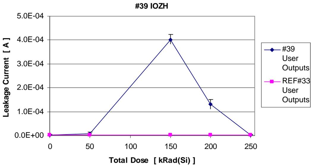
Figure 7.13 Average Output Leakage high Current for sn#39 for user I/Os. Measurement at 200 and 250 krad(Si) are the two annealing steps. All measurement over  $1.2 \times 10^{-4}$  A was made with another instrument. Error bars indicate max and min measured value for each device.
