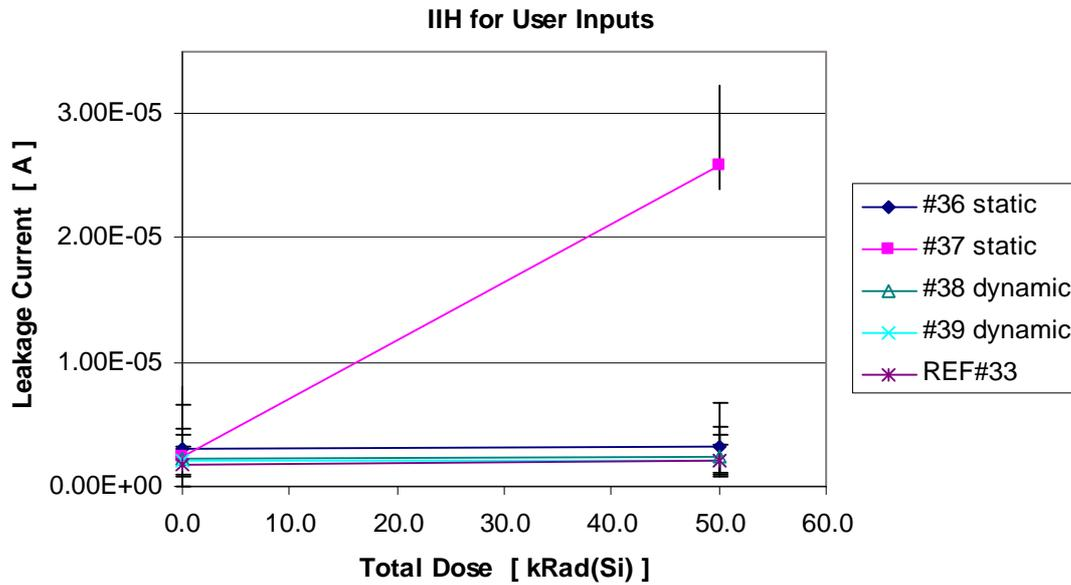
Figure 7.9 Average Input Leakage High Current for all measured user I/Os and devices up to 50krad(Si). Specification limit is  $1 \times 10^{-5}$  A. Error bars indicate max and min-measured value for each device.
