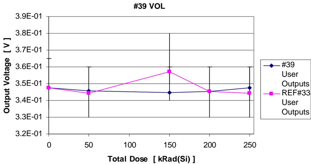
Figure 7.16 Average Output Low Voltage for SN#39 for user I/Os. Specification limit is 0.4 Volts but the parameter is measured at nominal supply voltage conditions. Pre-irradiation measurement was performed with specified these conditions and are not presented since it isn't valid for comparison. Error bars indicate max and min measured value for each device. Measurement at 200 and 250 krad(Si) are the two annealing steps.
