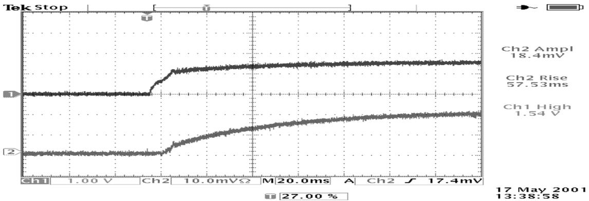
Figure 7.6 Oscilloscope image of  $V_{CCINT}$  (Ch1- 1V / div) and  $I_{CCINT}$  (Ch2- 1.0A / div) for sn#37 after 50krad(Si) (20ms / div). The device was never initialised likely because of the current limit at 2A on the power supply.
