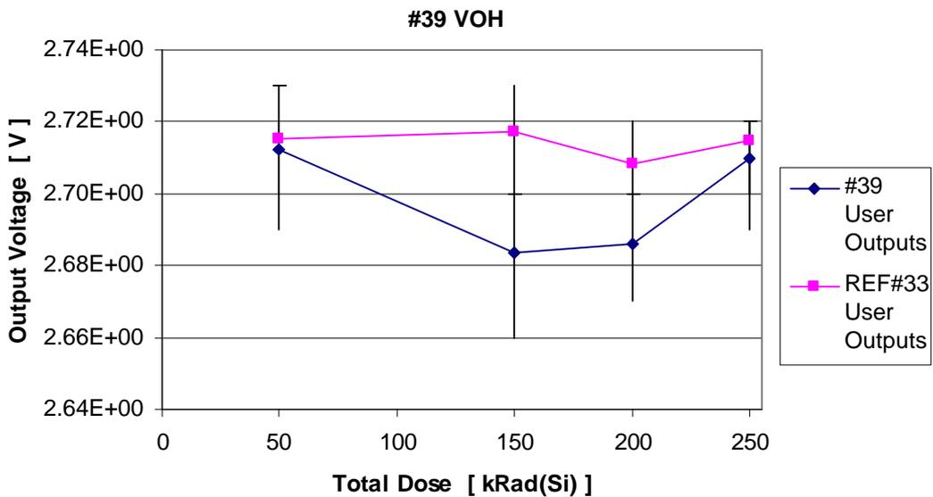
Figure 7.15 Average Output High Voltage for SN#39 for user I/Os. Specification limit is 2.4 Volts but the parameter is measured at nominal supply voltage conditions. Pre irradiation measurement was performed with specified these conditions and are not presented since it isn't valid for comparison. Measurement at 200 and 250 krad(Si) are the two annealing steps. Error bars indicate max and min measured value for each device.
