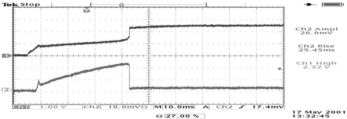
Figure 7.5 Oscilloscope image of  $V_{CCINT}$  (Ch1- 1V / div) and  $I_{CCINT}$  (Ch2- 0.5A / div) for sn#36 after 50 krad(Si) (10ms / div). The current peak observed in the pre-irradiation case is here followed by further increase in the current until the voltage has reached 1.2V.
