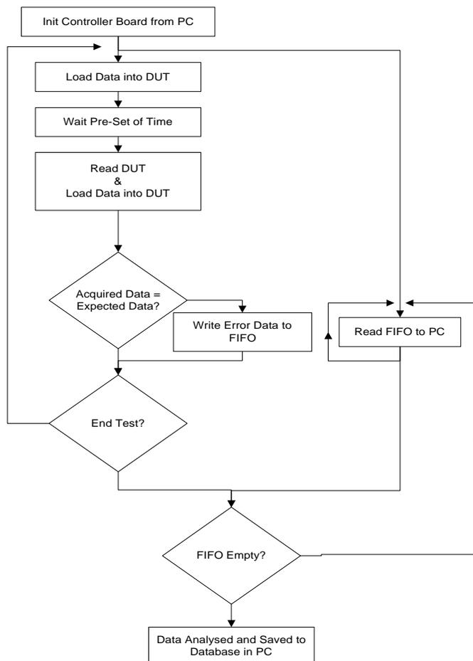
Figure 4.1 Flow chart of the test sequence.
