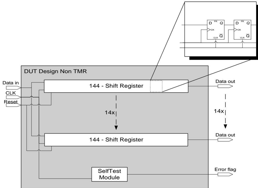
Figure 3.2 Principal Drawing of part used for functional test in the Non-TMR DUT Design.
