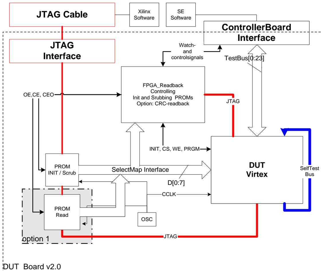
Figure 4.3 Schematic drawing of DUT board with configuration interface for the Virtex device.
