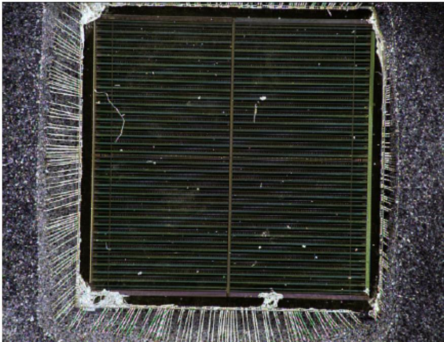
Figure 3.1 Overview of Virtex XQVR300 chip. Chip size is 11,2 x 11,2 mm.
