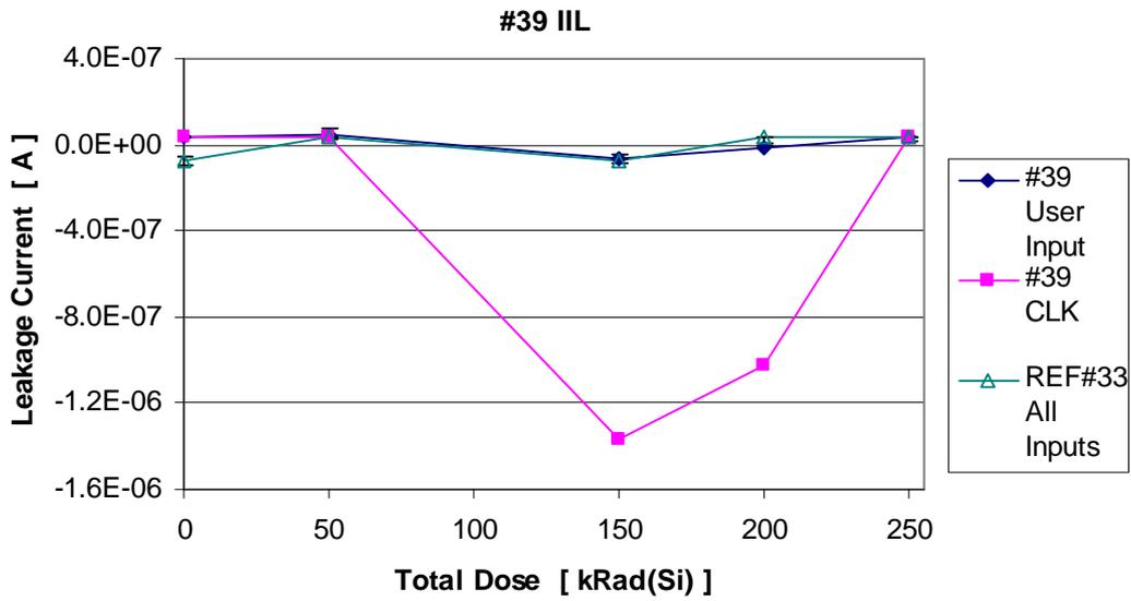
Figure 7.12 Average Input Leakage Low Current for sn#39 for user I/Os and dedicated Clock. Measurement at 200 and 250 krad(Si) are the two annealing steps. All measurements are well within specification limit of  $1 \times 10^{-5}$  A. Error bars indicate max and min measured value for each device.
