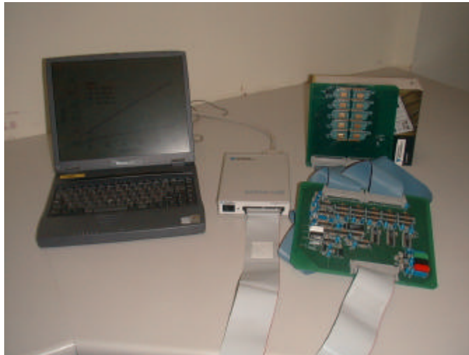
Figure 3: The complete RADFET Reader Board (RRB) system comprises (from left to right): a PC running a dedicated LabView program; Data Acquisition Card (DAC); RADFET Reader Control Board (RRCB) – down, and RADFET Socket Board (RSB) – up. The PC and DAC are outside the radiation room, RRCB is inside the room but shielded against radiation, and RSB with the RADFETs mounted on it is exposed to radiation.
