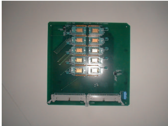
Figure 5: The RADFET Socket Board (RSB). The two 50-way connectors at the bottom provide connection with RRCB. The 10 RADFET sockets have RADFET chips mounted on them. The size of the area with RADFET chips is 10cm x 5cm. There are two temperature sensors: top left and down right from the RADFET chip area.
