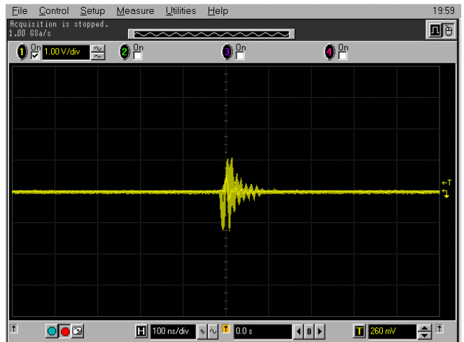
Figure 6-28: Run 26, SET Effects on CLC501 Appl. B (68 MeV cm 2 /mg, pulse height: 1.1V, pulse width: <100ns )
