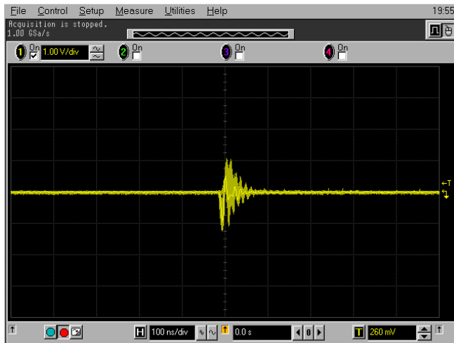
Figure 6-27: Run 25, SET Effects on CLC501 Appl. B (48.04 MeV cm 2 /mg, pulse height: 1V, pulse width: <100ns )
