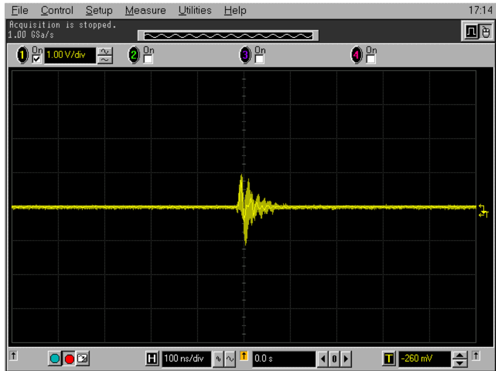
Figure 6-29: Example for "negative" SETs, CLC501 Appl. B, LET=14.1 MeV cm 2 /mg, 454 events, 0° tilt angle (Run 12, pulse height: -1.1V, pulse width: <100ns )
