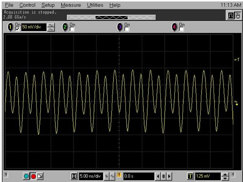
Figure 6-48: Oscillation on \mu PC2712B arrangement at UCL
