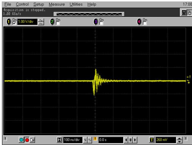
Figure 6-25: Run 9, SET Effects on CLC501 Appl. B (28.2 MeV cm 2 /mg, pulse height: 0.9V, pulse width: <100ns )
