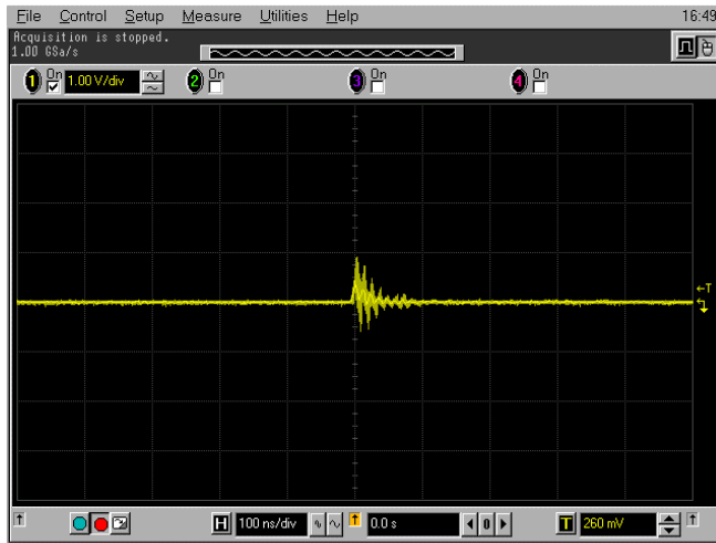
Figure 6-14: Run 8, SET Effects on CLC501 Appl. A (28.2 MeV cm 2 /mg, pulse height: 0.9V, pulse width: <100ns )
