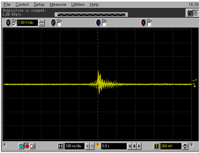
Figure 6-12: Run 6, SET Effects on CLC501 Appl. A (14.1 MeV cm 2 /mg, pulse height: 1V, pulse width: <100ns )
