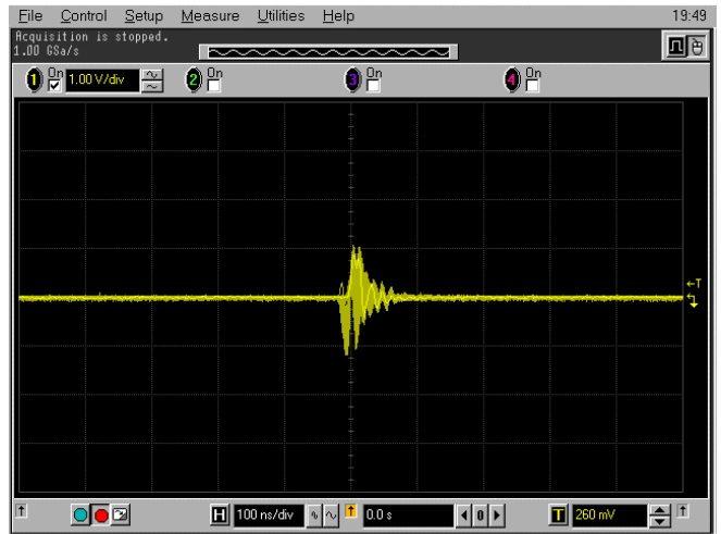
Figure 6-26: Run 24, SET Effects on CLC501 Appl. B (34 MeV cm 2 /mg, pulse height: 1V, pulse width: <100ns )
