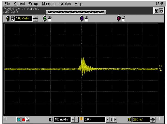
Figure 6-15: Run 23, SET Effects on CLC501 Appl. A (34 MeV cm 2 /mg, pulse height: 1.05V, pulse width: <100ns )
