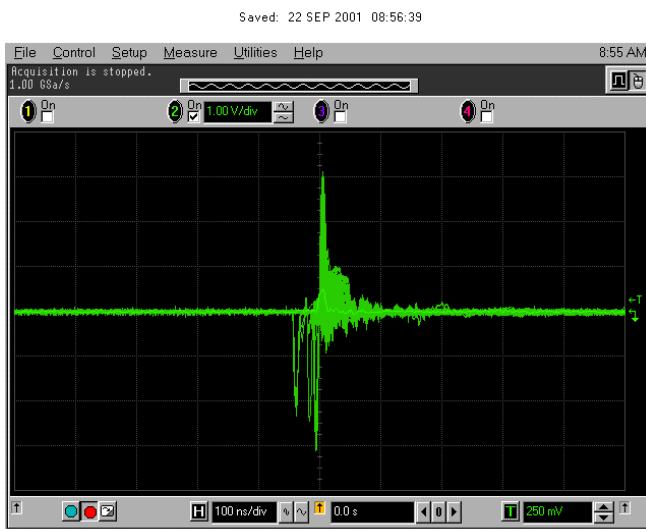
Figure 6-41: Run 28, SET Effects on CLC505 (48.08 MeV cm 2 /mg, pulse height: 3.2V, pulse width: <100ns )
