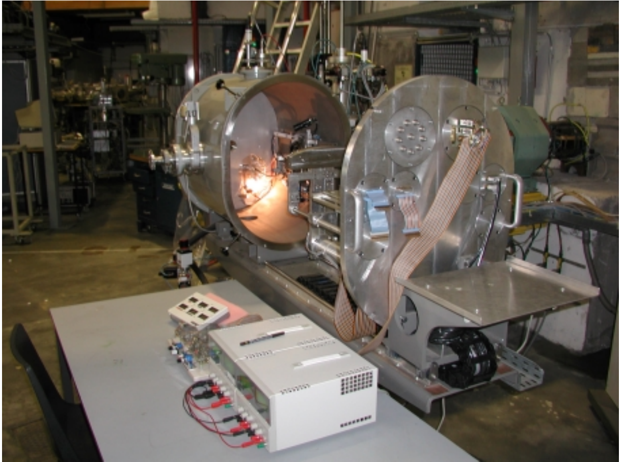
Photograph 1 – Open irradiation chamber with mother and daughter boards mounted inside open door, and biasing and monitoring circuitry on table in foreground
