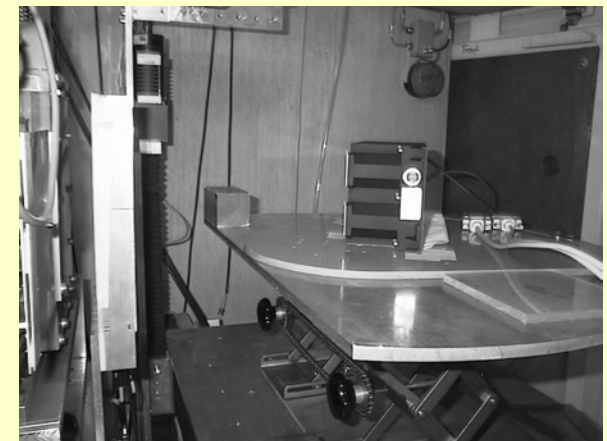
SREM unit placed on the angular stage (and two plastic detectors in front - up)
