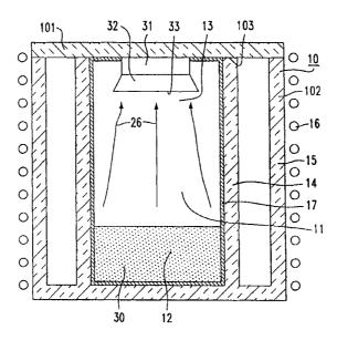
(11) containing a storage area (12) for a solid SiC supply (30) and a crystal area (13) wherein the SiC monocrystal (32) is grown on a SiC seed crystal (31). One side of the crucible (11) facing the inner area thereof is covered with a film made of tantalum, tungsten, niobium, molybdenum, rhenium, iridium, ruthenium, hafnium or zircon, whereby the crucible is sealed and aggressive constituents of the SiC gaseous phase are prevented from reacting with the wall of the crucible.
