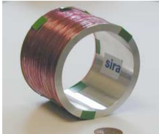
Figure 1.2.2-1 Al fibre bobbin with fibres for proton irradiation
