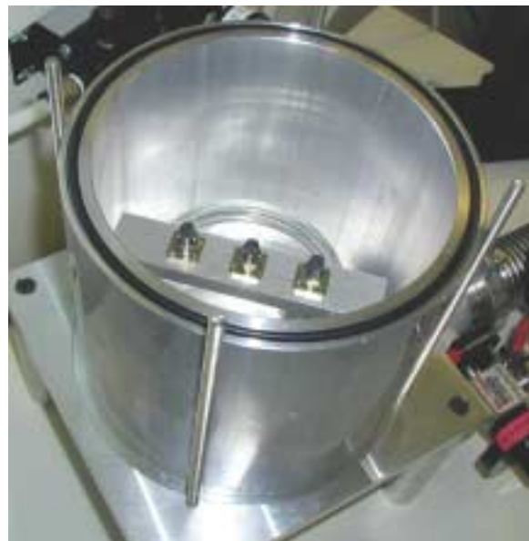
Figure 1.3-5 Mounting Base-Plate For Testing Optical Fibre Connectors
