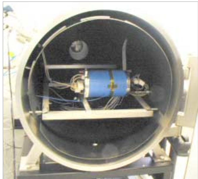
Figure 1.5-5 Cable Support Cylinder Mounted Within Siras Thermal-Vacuum Chamber
