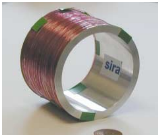
Figure 2.2-1 Fibre bobbin with fibres for proton irradiation
