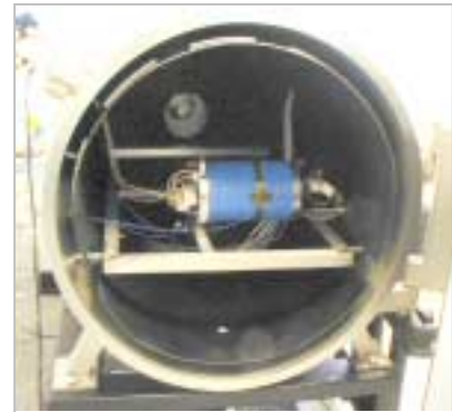
Figure 5.3-3 – Cable Support Cylinder in Thermal Vacuum Chamber
