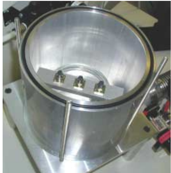
Figure 5.1-3 - Mounting Base-Plate For Testing Optical Fibre Connectors
