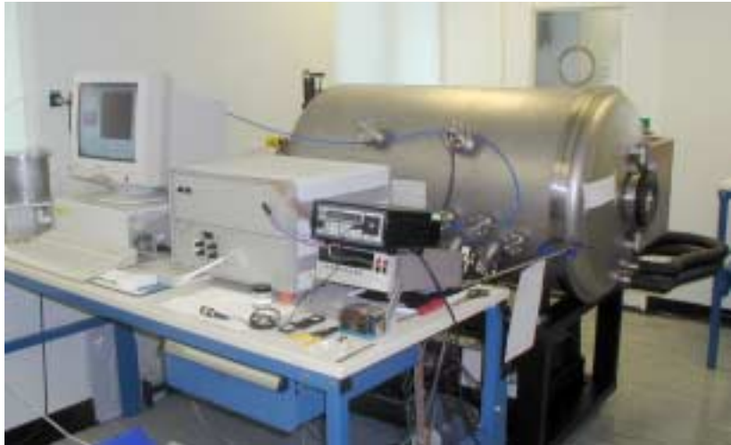
Figure 5.3-1 - Thermal Vacuum Test Facility
