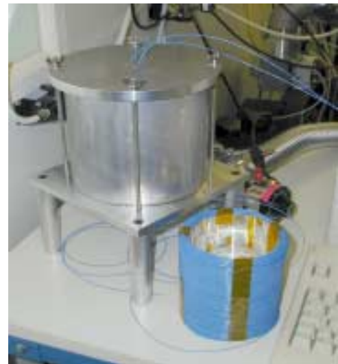
Figure 5.1-2 - Test Cable On Flexible Former
