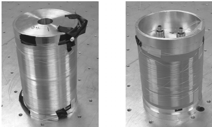
Fig. 1. Pictures of the spools used for the irradiation tests. The spool on the left is used for the room temperature test and the spool on the right can be temperature-controlled.
